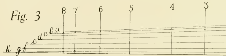
PRICKING OFF CORNER PILLAR ON TWISTED OR WINDING SURFACES OF A LANDAULET BODY WITH JOINT IRONS.
