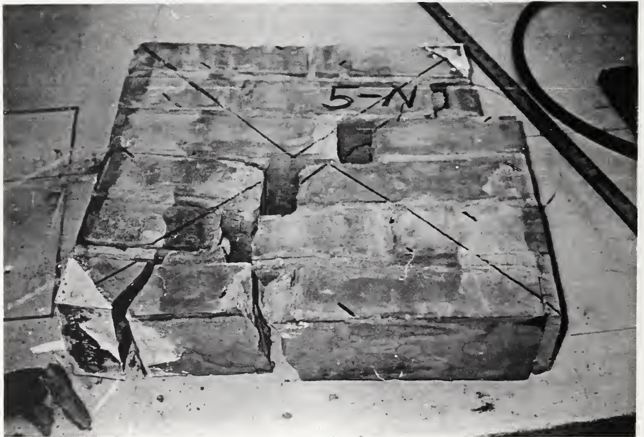
Figure 5.10.4. Diagonal tension specimen taken from Office Building
