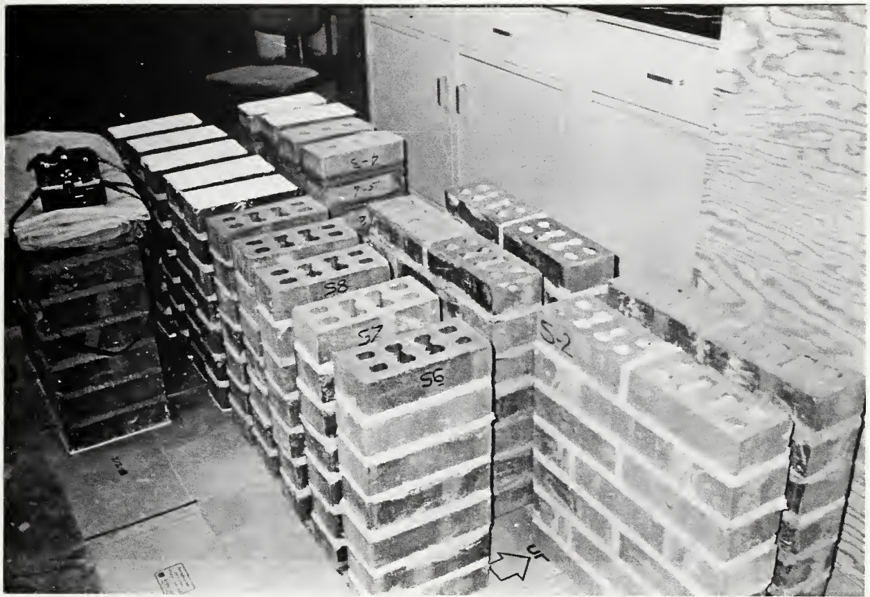
Figure 5.10.3. Laboratory-built prism and panel specimens
