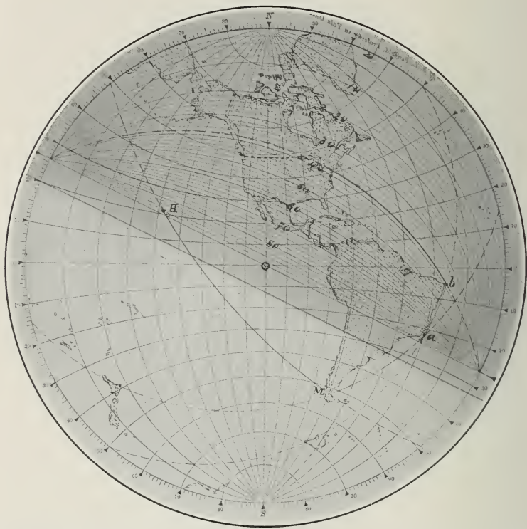
Stereographic Protractor adjusted for finding the great circle track from b to New York. Other great circles, H to M , M to a and a to b , have been drawn on the map. Great circles only are printed on the protractor.
