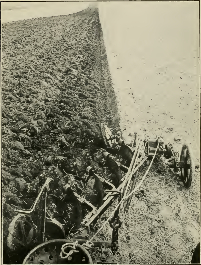
Tractor disk plow showing the way the disk plow turns the soil and also that a straight furrow can be turned with one of these implements.
