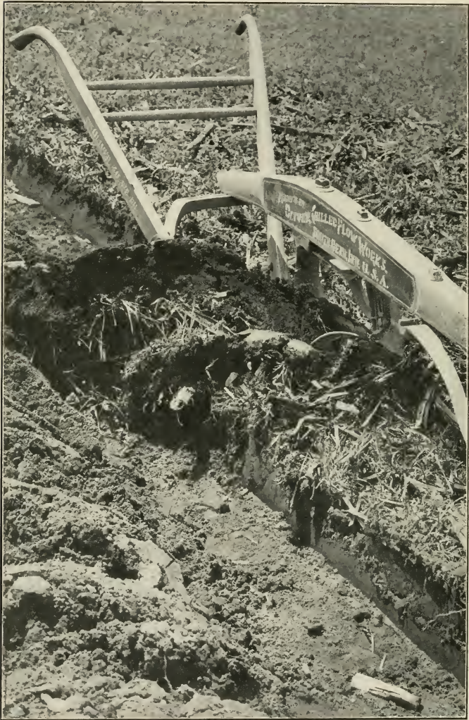
Observe the jointer turning a little furrow into the right-hand corner of the big furrow bottom. This is necessary for ideal plowing.
