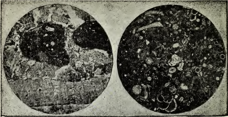
Figs. 4 and 5.—Structure of Melbourn Rock and of Chalk Rock (magnified fifty times).
