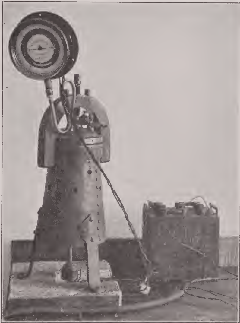
FIG. 46.—Autoclave for testing valves and packing in steam under high pressure
