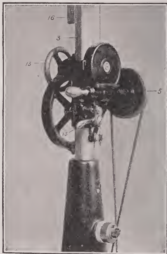
FIG. 26.—Detail of lower portion of machine shown in Fig. 24, illustrating stepped pulley, gear drive, and releasing mechanism
