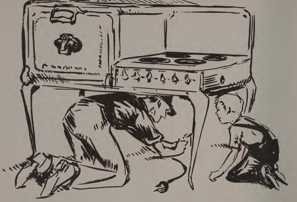
Sparks installed a separate circuit for the electric stove. This used 220 volts. The lights in the house used only 110 volts. He used heavy wire for this circuit. He connected the stove by a heavy plug in the base board. He explained what caused the stove to heat. When the electric current flows through a wire that resists the current the wire gets hot.
