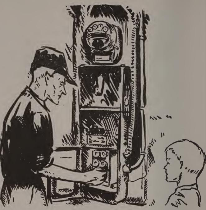
used in the house. He installed a switch box so that all the lights in the house can be turned out. He put in a fuse box. There was a fuse for each circuit. If anything went wrong with any circuit it would blow the fuse in that circuit and not hurt the wiring.
