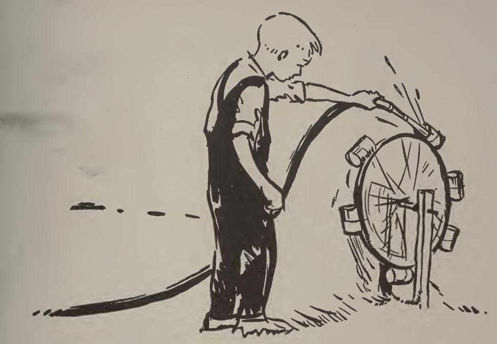
When Little Sparks came home he made a little turbine. He fastened small tin cans to the rim of an old cartwheel. He held the garden hose so that it squirted into each can. The water dumped out of each can as it came to the bottom. The wheel whirled around and around.
