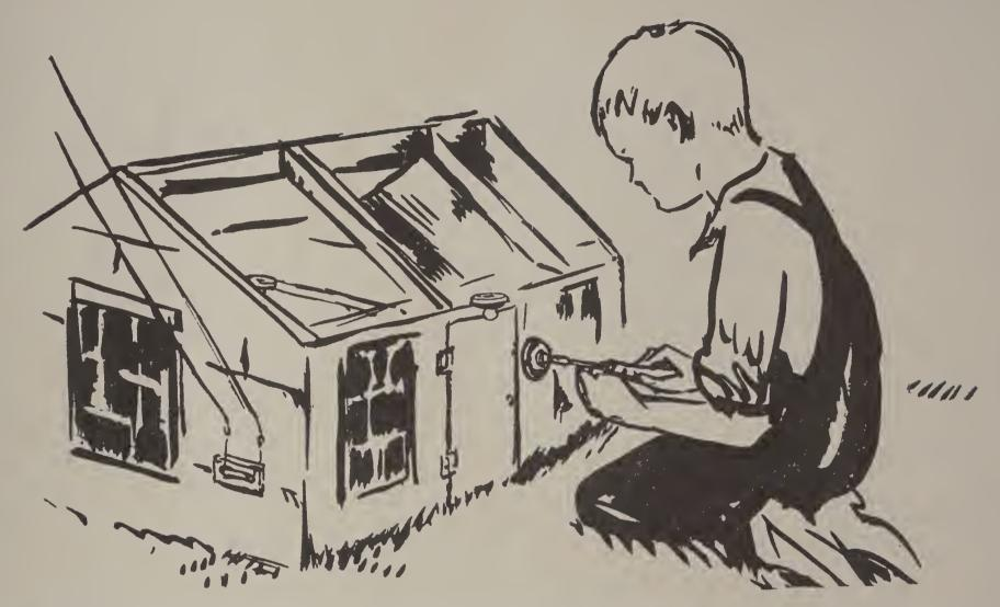
Little Sparks got a pushbutton and a buzzer from Sparks. Sparks showed him how to connect these into his battery circuit. He ran a wire from his switch to the pushbutton. He ran a wire from the pushbutton to the buzzer. He ran another wire from the buzzer to the wire outside the playhouse which was not connected to the switch. When he pressed the button the buzzer sounded.
