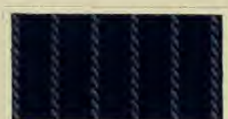
Dyed with: 6% Benzo Chrome Black Blue B; Printed with: zinc white.
