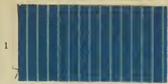
Dyed with: 1% Benzo Sky Blue; Printed with: zinc white.
