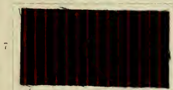
Halfwool dyed with: 6% Direct Deep Black G, 1% Sulphon Cyanine G B extra, 1/2% Sniphan Blue Black; Discharged with: 6% Rhodamine 6 G and 0.8% Auramine II.
