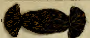
1 Dyed with: 6% Benzo Chrome Black Blue B; Discharged with: 4% Auramine G.
