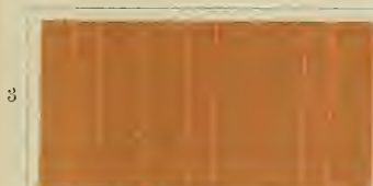
Dyed with: 5% Benzo Purpurine 4 B; Printed with: zinc white.
