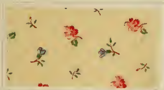
Chloramine Orange G padded on colour prints.
