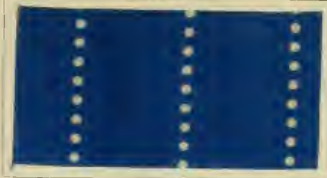
Dyed with: 2% Brilliant Benzo Blue 6 B; discharged with tin.
