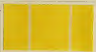
Dyed with: 2% Chrysophenine; discharged with tin.
