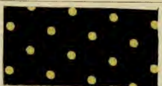
Aniline Black discharged with Chloramine Yellow.
