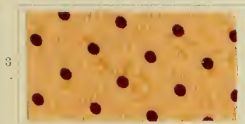
Dyed with: 0.1% Congo Orange R; Discharged with: 2% Rhoduline Violet.
