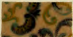
Dyed with: Benzo Purpurine 1 B; discharged with: Methyl Violet, Brilliant Green, Persian Berry Yellow.
