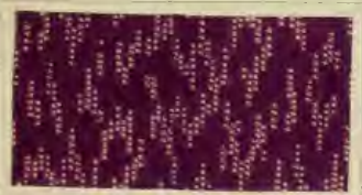
Dyed with: 6% Benzo Violet R; discharged with tin.
