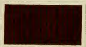
Halfwool dyed with: 2% Benzo Chrome Brown B, 0.4% Benzochrome Brown G; Discharged with: 1.5% Brilliant Green crystals and 1.5% Auramine G.
