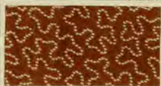
Dyed with: 4% Benzo Chrome Brown R; discharged with tin.
