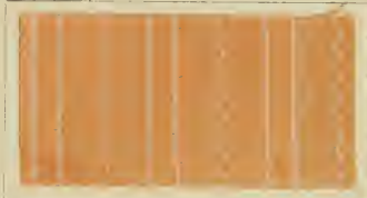
Dyed with: 5% Brilliant Purpurine R; discharged with zinc powder.
