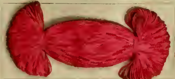
10 Printed with: Caustic Soda; Dyed with: 2% Brilliant Geranine B.
