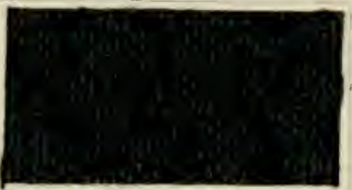
Aniline Black; dyed with 1 1/2% Chrysofenine and 1 1/2% Brilliant Benzo Blue GB.
