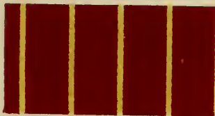
Ice Bordeaux padded with Chloramine Yellow.
