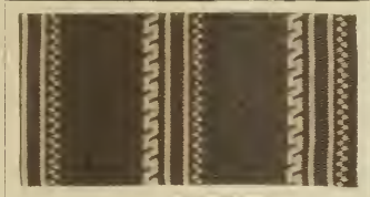
Dyed with: 5% Benzo Brown BX; discharged with zinc powder.
