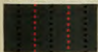
Dyed with: 3% Benzo Green G; discharged with: 3% Rhodamine 6G; printed with: 30% Fast Black.
