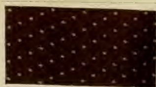
Dyed with: 4% Benzo Chrome Brown B; discharged with tin.
