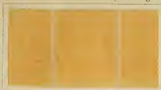
Dyed with: 2% Congo Orange G; discharged with tin.
