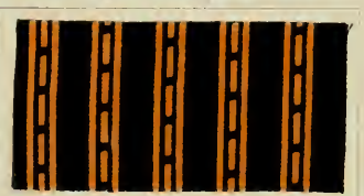
Aniline Black discharged with Congo Orange G.
