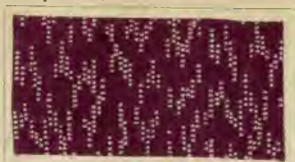
Dyed with: 4% Azo Violet; discharged with zinc powder.
