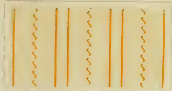
Wool printed with: 2% Benzo Orange R.
