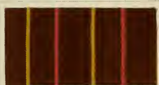
Dyed with: 3% Benzo Chrome Brown R; discharged with: 3% Rhodamine 6G, Persian berry Yellow discharge.
