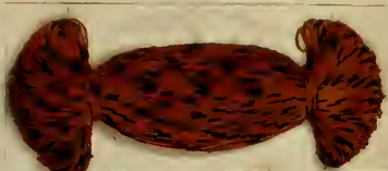
2 Dyed with: 3% Benzo Chrome Brown G; Discharged with: 1% Methyl-Violet 6 B.
