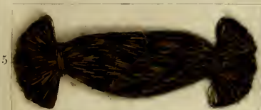
5 Dyed with: 8% Pluto Black B; Discharged with: 4% Auramine G.
