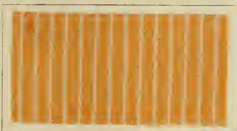
Dyed with: 2½% Congo Orange R; discharged with zinc powder.
