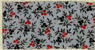
Benzo Chrome Black Blue B padded on Aliz. Red and Aniline Black.
