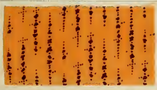
Dyed with: 3% Congo Orange B. Cover printed with: 1/2% Methyl Violet 2 B.
