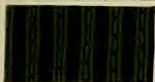
Dyed with: 8% Direct Deep Black T; discharged with: 2.5% Auramine G, 0.5% Brilliant Green crystals.
