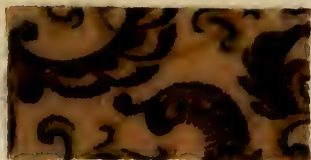
Dyed with: Benzo Purpurine 4 B; discharged with: Persian Berry Yellow and Methyl Violet.
