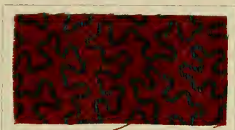
Dyed with: 2% Benzo Chrome Brown R; discharged with: 1½% Methylene Blue BB.
