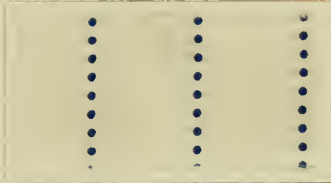
Half Silk printed with: 1% Brilliant Benzo Blue 6 B.
