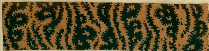
Dyed with: 4% Benzo Purpurine 4B; discharged with: 2% Brilliant Green.
