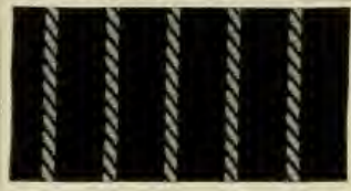
Dyed with: 8% Pluto Black B; discharged with tin.
