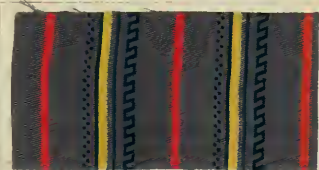
Dyed with: 1% Benzo Grey S extra; discharged with: 3% Rhodamine 6G, 2% Brilliant Green, Persian berry Yellow discharge.
