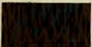
Dyed with: Benzo Brown NB and Geranine G; discharged with: Methylene Blue and Brilliant Green.
