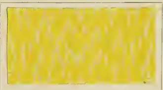
Dyed with: 2% Chrysophenine; discharged with zinc powder.
