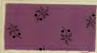
Aniline Black; dyed with 1% Heliotrope BB.
