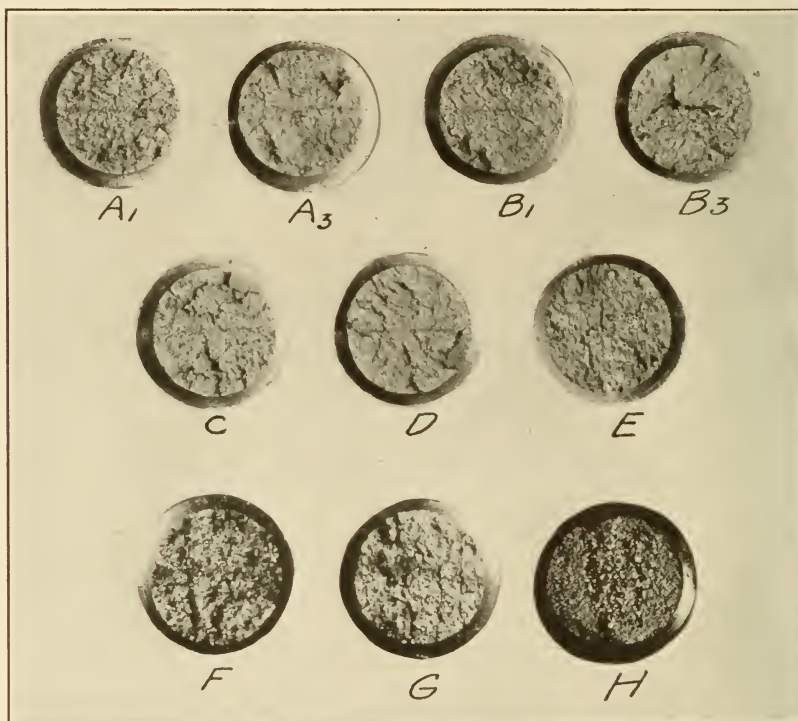
FIG. 4.—Typical fractures of iron broken by repeated impact (Eden-Foster test).
