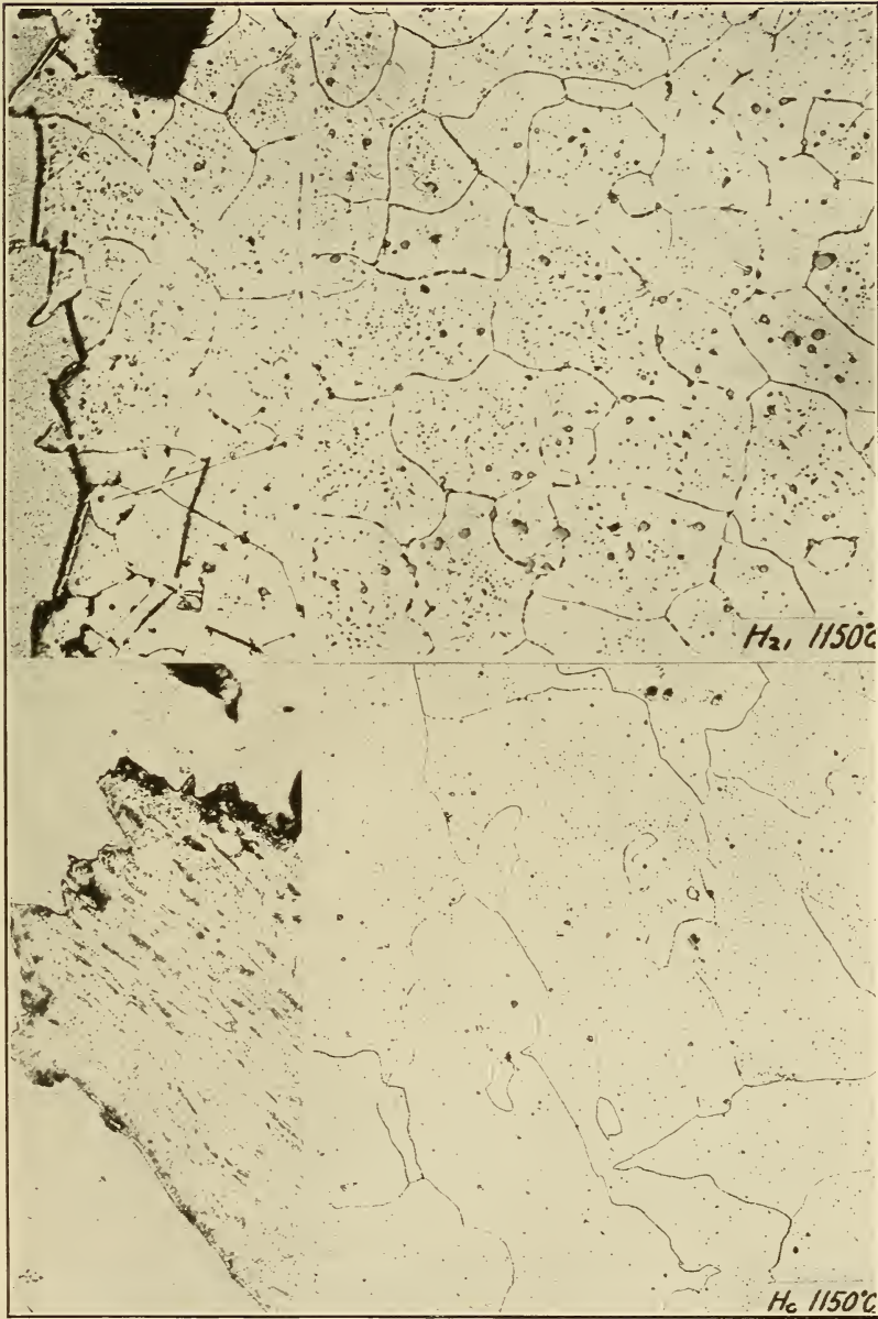
FIG. 22.—Relation of impact fractures of ferrite (open-hearth iron) to microstructure; initial magnification, \times 100 , slightly reduced.
