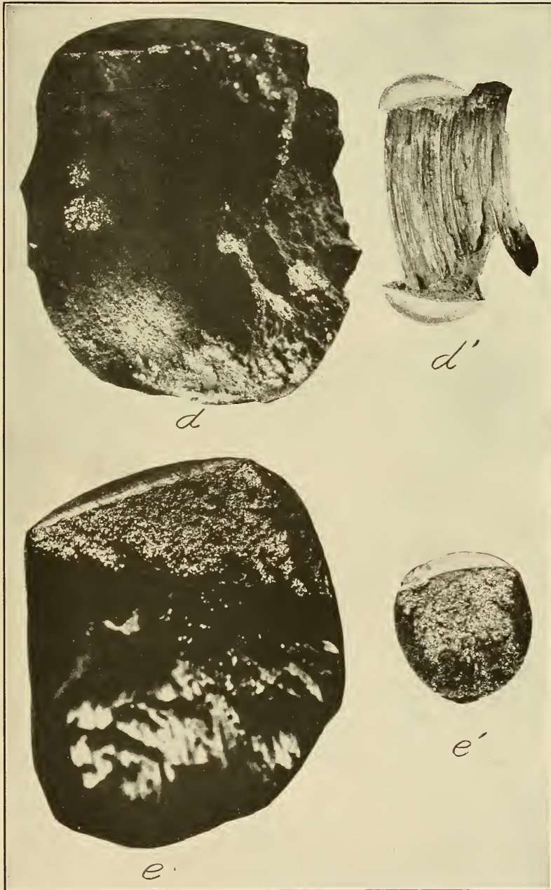
FIG. 15 (Continued).—Typical results obtained by the nick-bend test upon wrought iron, specimen G ( \times 1 ).
