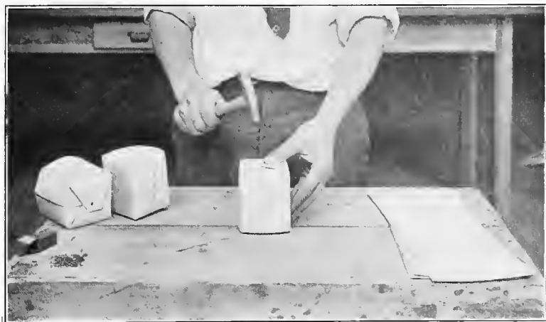
FIG. 11. — Driving a small tack through the folds of paper and over the end of a bolt that extends through the block.
