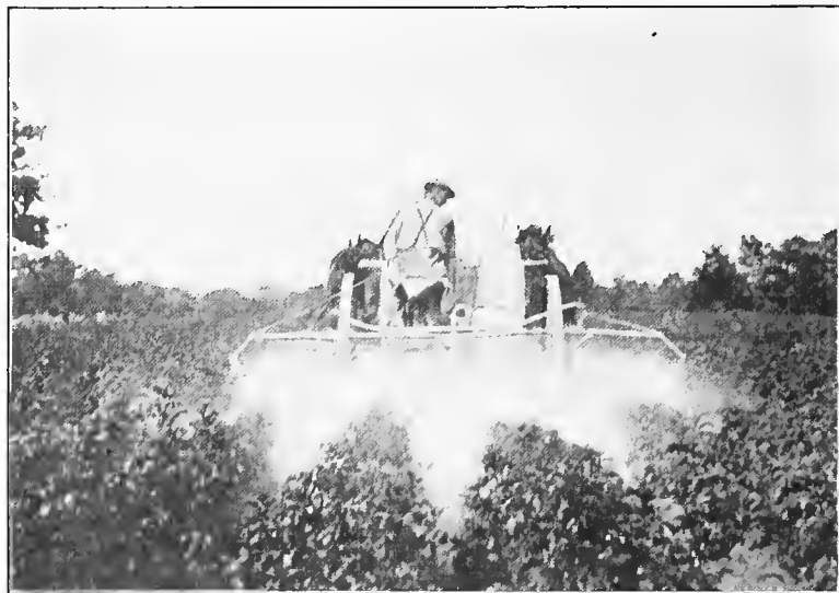
FIG. 56.—A spraying machine doing effective work. High pressure (200 pounds), proper nozzle adjustment, and plenty of material (100 gallons to the acre).
