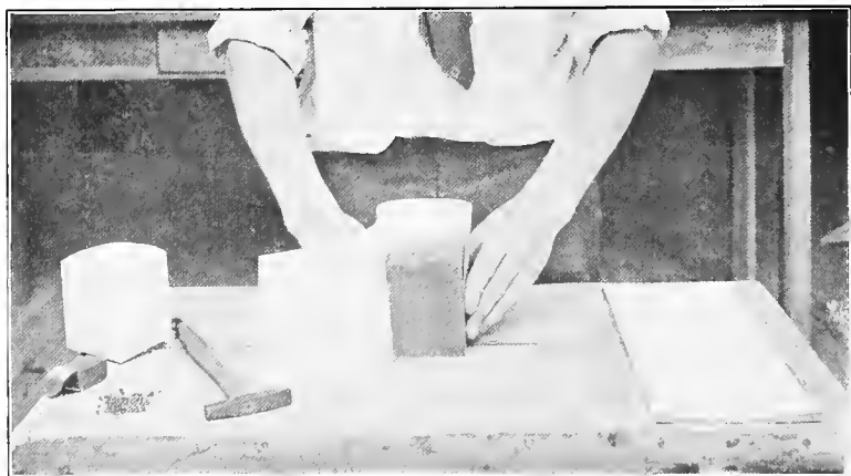
FIG. 9.— Folding the paper around the block which is secured to the bottom of a flat.
