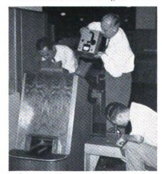
X-ray machines are being used in stores as shoe-fitting devices. The measuring devices used are an "r" condenser and an ion chamber. At the point where the feet are inserted is a 25-roentegen chamber. Few machines have adequate protection.
