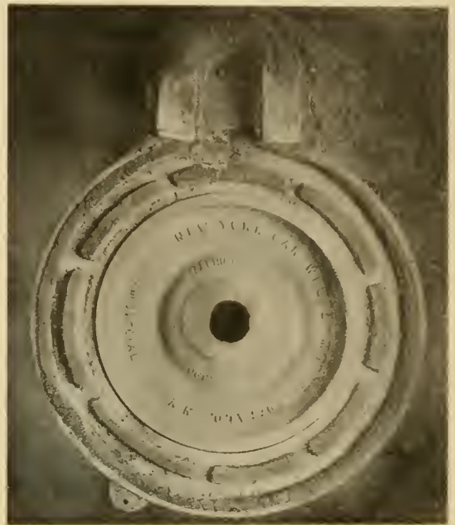
33-inch, 650-lb. Special Wheel After Thermal Test.
