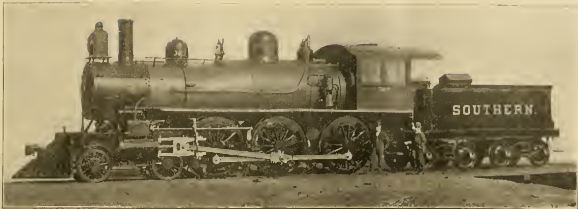
Ten-Wheel Passenger Locomotive—Southern Railway.
