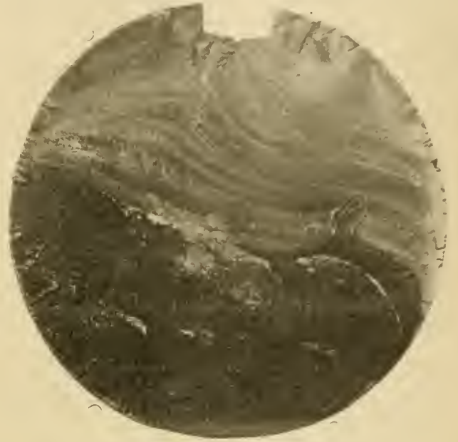
Photograph of Fractured Axle.
