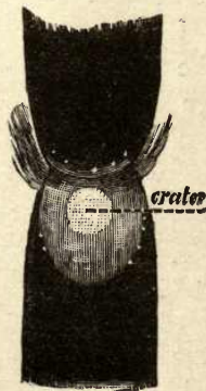
FIG. 2.—The Carbon Poles of an Electric Light.
