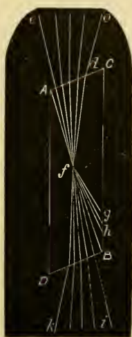
Path of the ordinary and extraordinary rays in a Nicol prism.
