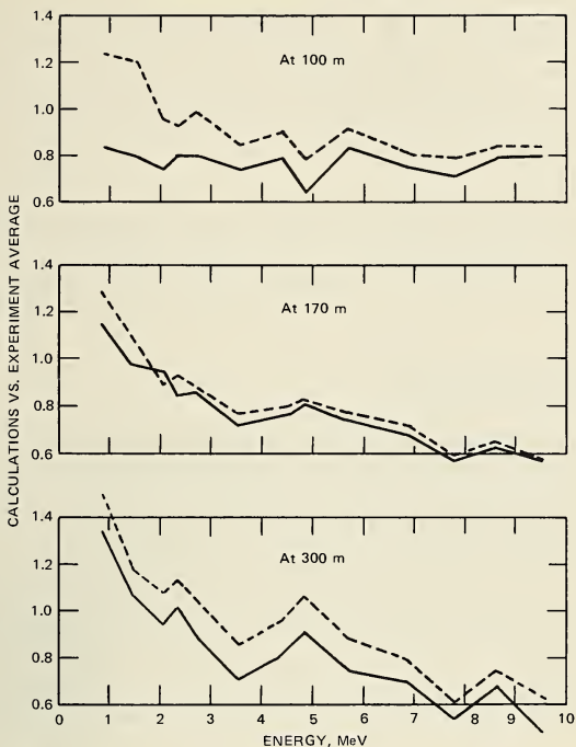
Fig. 5 Comparison of calculated spectra from Army Pulse Radiation Division (APRD) reactor. ---, LANL, Monte Carlo code (MCNP). —, Defence Research Establishment, Ottawa (DREO) DOT-3.
