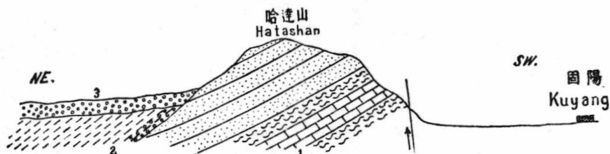
Fig. 10. Section N. of Kuyang. 1, Wutai quartzite and marble. 2, Tertiary red clay. 3, Gravel.
