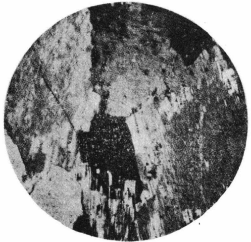
B. Gneissic granite—mainly orthoclase, microcline, perthite, hornblende and quartz; specimen from Miaoërhkou. \times 32 and N +
