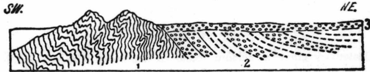
Fig. 27. Section about 15 li SE of Shihnakan. 1. Gneiss. 2. Red or green clay (Miocene-Pliocene). 3. Gravel.
