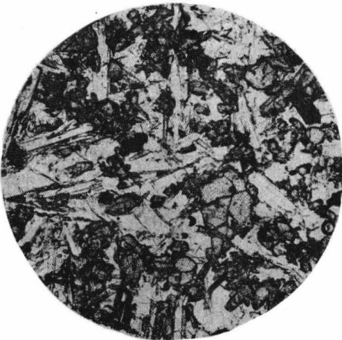
C. Coarse olivine diabase—lathes of colourless labradorite embedded in gray augite crystals, showing the diabasic structure. Specimen from Hanoorpa formation near Huanghuakotung. \times 32
