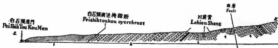
Fig. 19. Section along the valley of Peishihtoukou, Kueisui (after C. C. Wang). 1, Sangkan system. 2, Permo-Triassic red shale and sandstone. 3, Lower Jurassic coal series. 4, Middle and Upper Jurassic red shale and sandstone.
