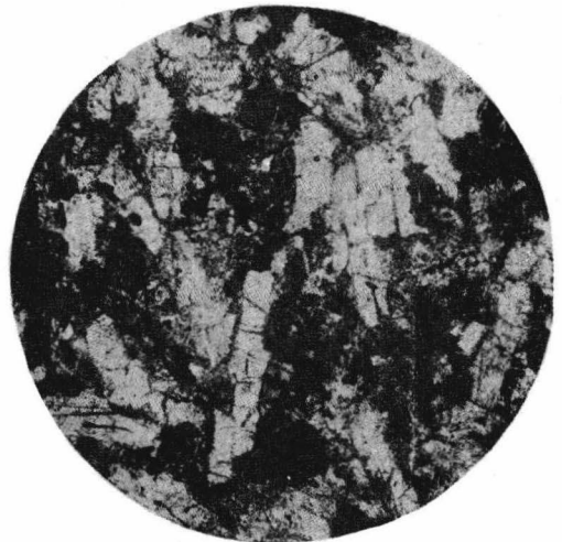
D. Diabase—Diabasic structure of augite mass, enclosing lathes of plagioclase. Specimen from basic intrusive in Sangkan system, T'sainaopao. \times 32
