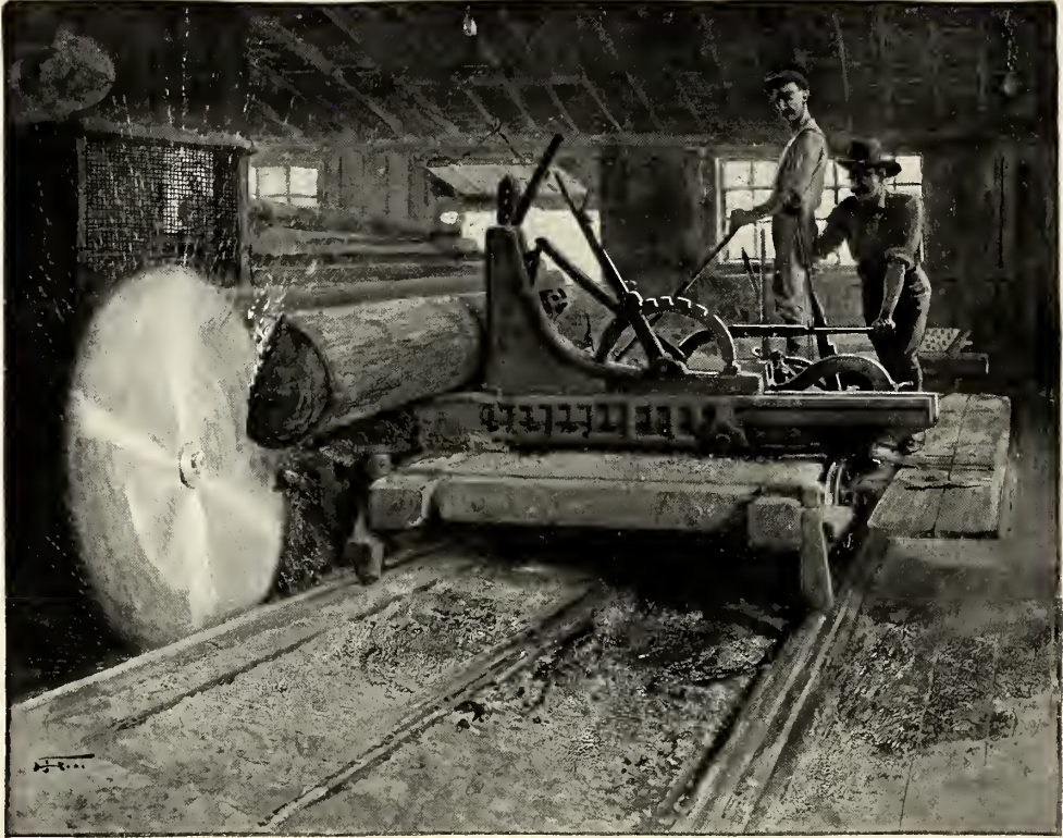
THE CIRCULAR SAW AT WORK, SHOWING THE CARRIAGE BEARING THE LOG.
