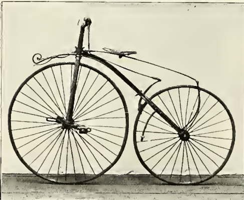
TENSION-WHEELED BONESHAKER, METAL RIMS AND RUBBER TIRES. THE "MISSING LINK" BETWEEN THE BONESHAKER AND THE ORDINARY. 1870.
