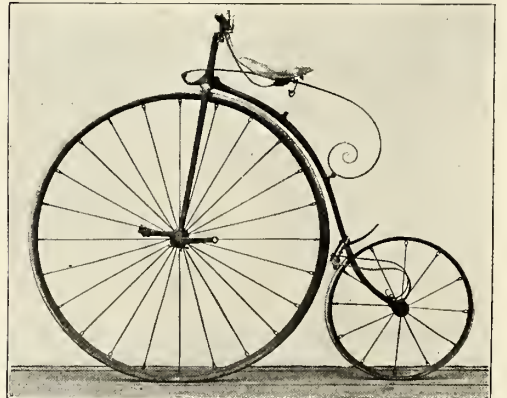
GROAT'S TENSION. ONE OF THE FIRST (AND BEST) RUBBER-TIRED TENSION-WHEELED BICYCLES PUT ON THE MARKET; NOTE DOUBLE STEP AND JOINTED BOW-SPRING; BRAKE CORD, ACTING ON HIND WHEEL, IS BROKEN.
