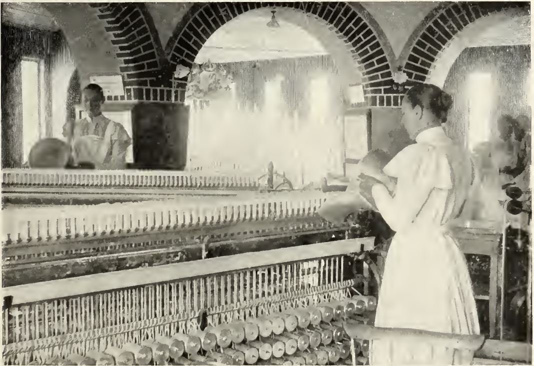
IN A SWEDISH CANDLE-FACTORY. FILLING THE MOLDS WITH MELTED STEARIN.
