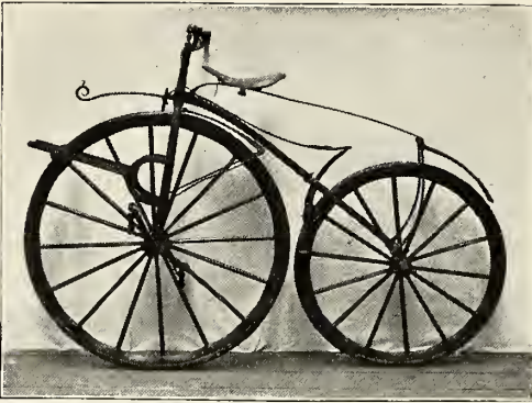
THE "BECK"; WOODEN WHEELS AND LARGE RUBBER TIRES. 1869 OR 1870.*
