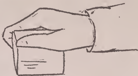
Fig. 20. Keep the wax or chalk thin on the edge and hold it firmly in marking around the pattern
