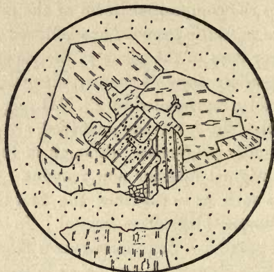
FIG. 4.—Aggregate of feldspar crystals showing the clear appearance of the microperthite in contrast with the clouded plagioclase.
