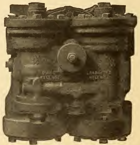
Fig. 109. Westinghouse "3-E" Control Valve, Showing Front View
