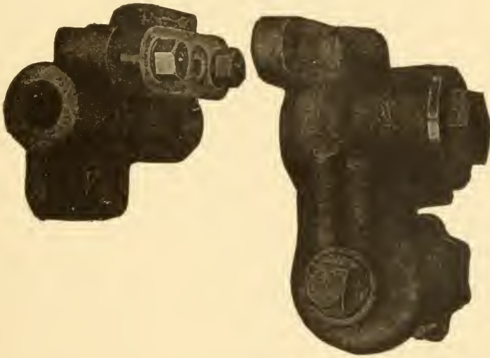
Fig. 38. "B-6" Feed Valve, Showing Valve Removed from Pipe Bracket
