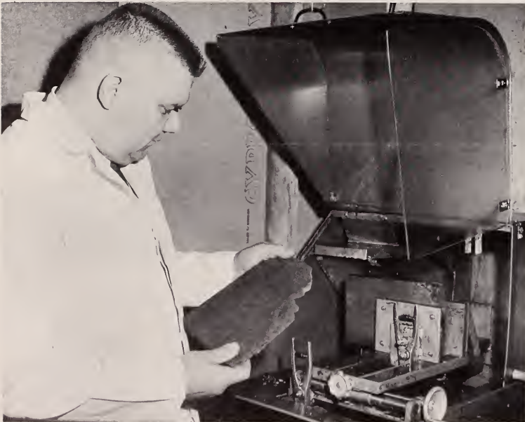
This fine piece of jasper has just been sawn off a larger block using the diamond bladed saw. The slab may then be cut up into smaller pieces to make costume jewellery or used for a larger item such as an ornamental desk set.
