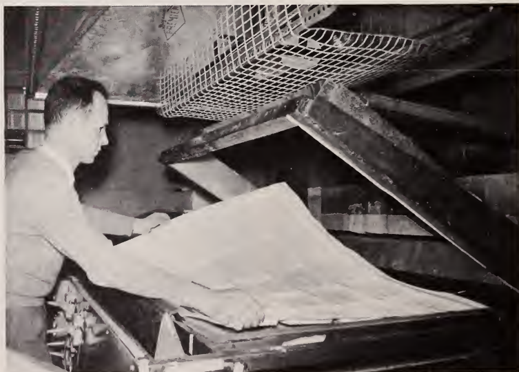
Plastic meat trays are moulded 25 at a time and separated after they are removed from the mould.
