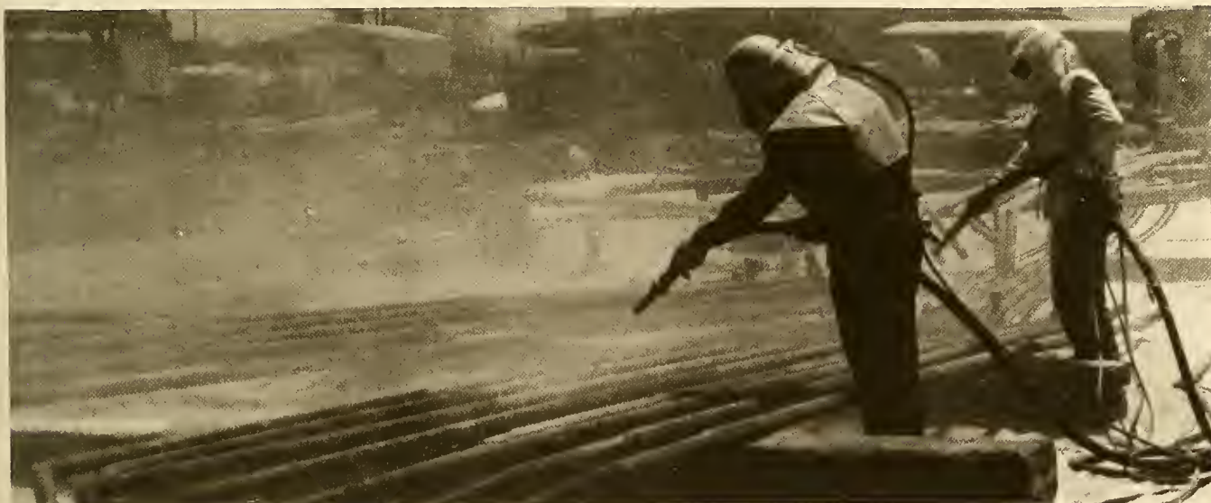
Many occupations pose a high risk for the development of lung disease. By wearing air supplied hoods, sandblasters above protect their lungs against inhaling the dusty atmosphere in a large steel fabrication yard.
