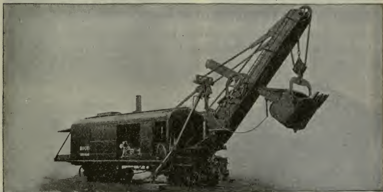
FIG. 1,634.—Bucyrus steam shovel for general contracting and railroad work in average materials.
