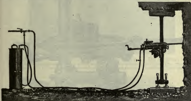
FIG. 1,373.—Leyner-Ingersoll drill set up on column, showing arrangement when water tank is used. Water under pressure is required and the pressure may be anything over twenty pounds and not higher than the air pressure. The water can be brought to the drill in any manner that is most convenient. Some run a small water pipe along with the air pipe, obtaining the supply either from outside the mine, or from the water in the mine, arrangements being made on the different levels so as to provide suitable average pressures. Others have one or more central tanks, each supplying several drills. In tunnel headings a suitable tank is often run in on a car. Where none of these methods is available a small individual tank for each drill is used. The tank usually employed weighs 70 pounds, is 3 feet 3 inches in height and 12 inches in diameter, and holds about 17 gallons. A smaller tank of about 6 gallons capacity can also be furnished, if preferred. Compressed air is admitted to the tank, and this forces the water to the drills under the same pressure as the air used to operate the drills, if taken from the same air line. The air which is admitted to the water tank is not the air which combines with the water and cleans the drill holes. This air comes from the drill. The water is carried from the water pipe line, or from the water tank, through a small water hose about 50 feet in length, then through a water regulating valve and a short piece of hose to the backhead of the drill. The water passes through the backhead plug and water tube, into the shank of the drill steel, where air from the drill mingles with it, and both pass on through the drill steel to the bottom of the drill hole. A swiveled connection is attached to the backhead, to which the short length of water hose is attached. The air hose is attached to the swivel connection at the valve chest. This method permits the hose to lie in a natural position close to the drill, and eliminates the necessity for a bend in the hose itself.
