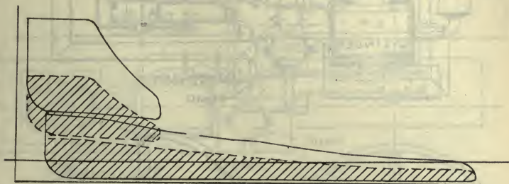
FIG. 1,177.—Actual combined diagrams illustrating regulation by throttling.
