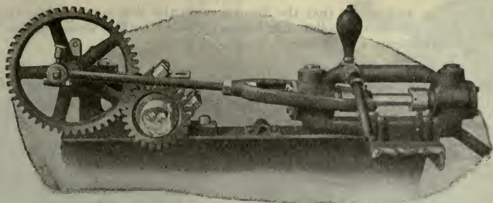
FIG. 1,740.—Case geared feed pump . It is driven by a gear on the crank shaft meshing with a larger gear that carries the crank pin which operates the pump. This pump has sufficient capacity to supply fifty per cent more water than needed by the boiler in extreme conditions. The feed water on its way to the boiler passes through the steel shell heater. By means of a by pass valve, the water can be returned to the tank when not needed in the boiler. The feed can be regulated making it unnecessary to stop the pump.
