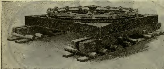
FIG. 1,631.—Semi-portable mounting consisting of rollers and skids.
