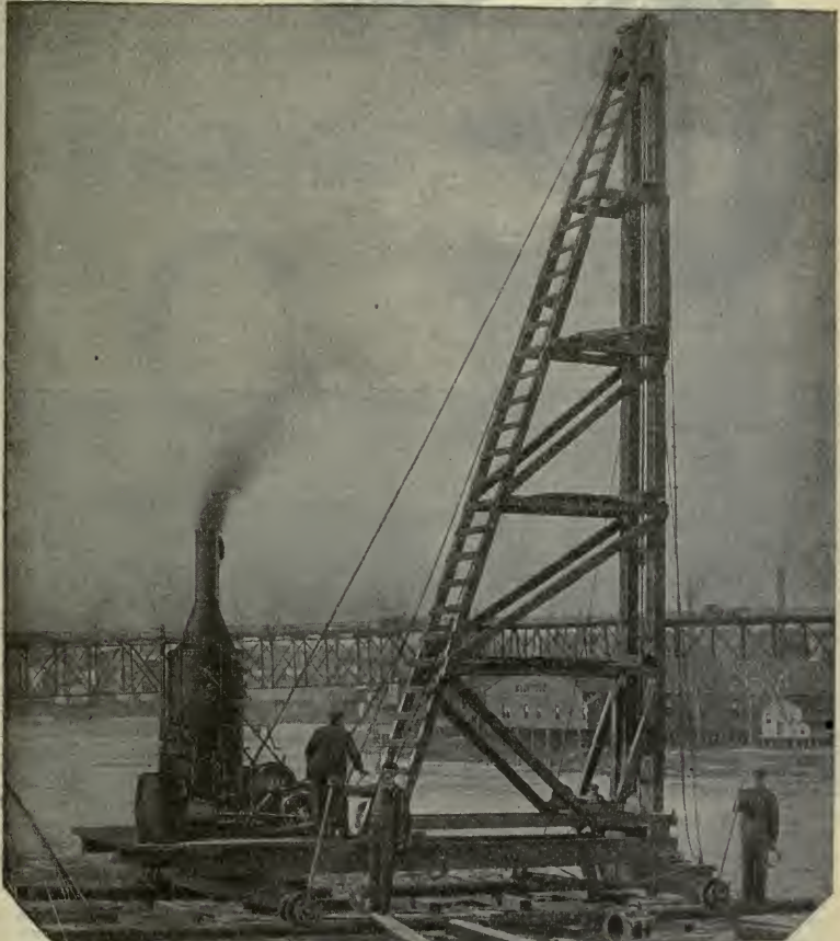
FIG. 1,607.—Mundy pile driver for land pile driving. The derrick is provided with a set of iron rollers bolted to the bed frame of the derrick. The rollers are made elliptical, for running lengthwise on a long wooden roller. The wooden rollers are heavily banded at the ends and arranged for moving the derrick sideways. This arrangement permits moving in any direction to suit the convenience of the work.
