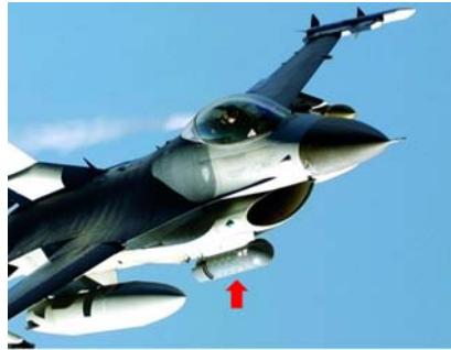
Figure 61. LITENING AT Targeting Pod Mounted Under the Air Intake of an F-16 522
