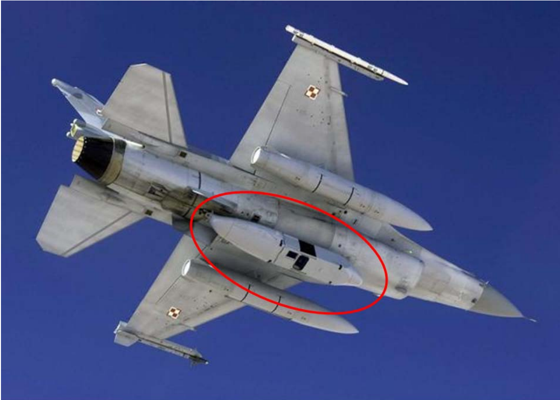
Figure 34. F-16 with Tactical Reconnaissance (TACRECCE) Pod on Center-line Mount (Circled in Red) 298
