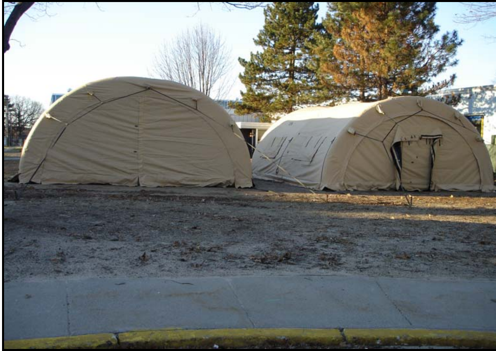
Figure 10. Non-insulated tent (left) and Aerogel insulated tent (right). Backside views of AirBeam TEMPER shelters. Evaluation conducted in Natick, MA.
