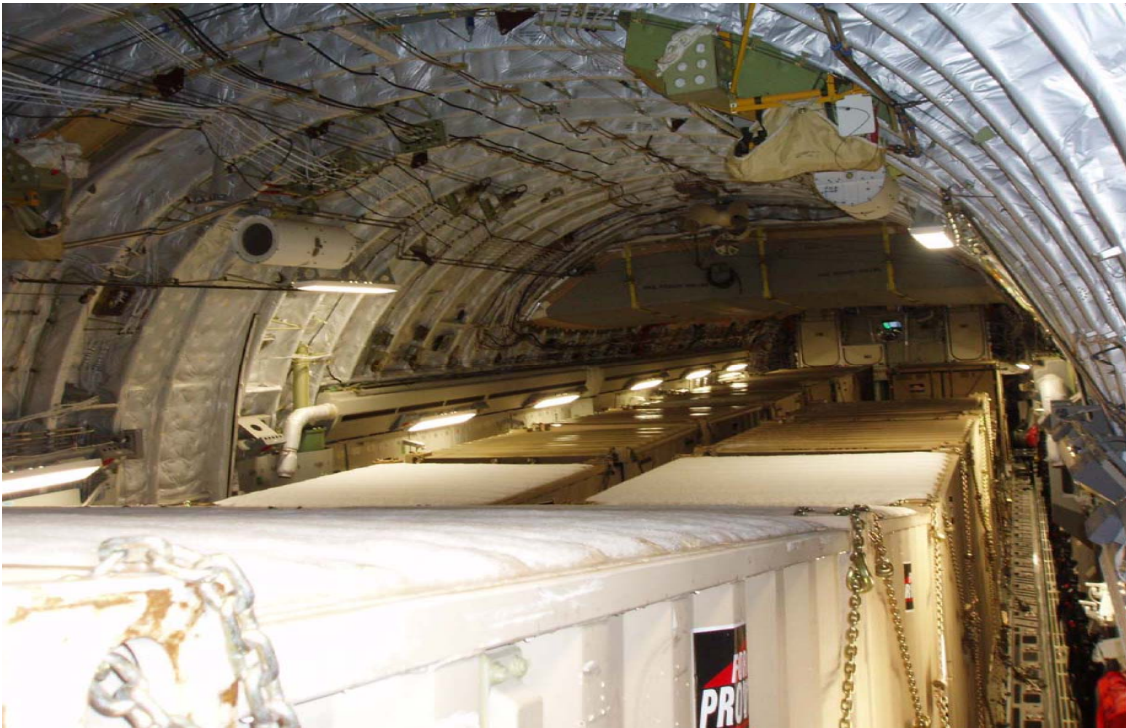
Figure 2. A complete EFPK Base Camp on one C-17 aircraft (18 pallet positions). Photo courtesy of Sustainment Division Materiel Systems Directorate Combined Army Support Command (CASCOM) November 2008.
