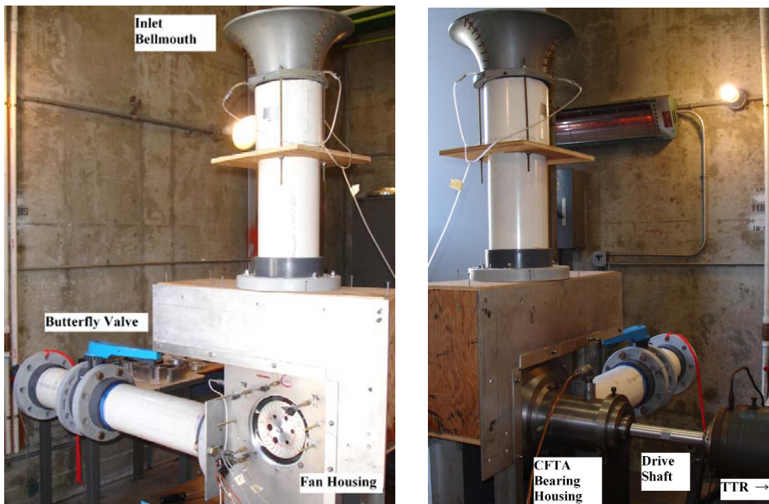
Figure 6. Cross-flow fan test assembly, (a) Front of CFTA with face plate removed from fan housing, (b) Back of CFTA, connecting to TTR
