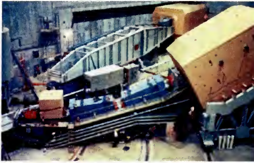
Figure 9: View of the End Station A spectrometer and detectors used to measure scattering from quarks within the proton and neutron. The scale is apparent from the human figure in the centre foreground.
