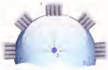
Figure 11. Combining the fibre output of an ICAN laser (Fig. 10) to a sphere (1) of more than 1m radius may produce a converging spherical laser pulse of 1ps duration and Exawatt power for interaction on a sphere 3 in the centre. Apart from diffraction limited beams with intensities above 10^{24} W/cm 2 for the application of HB11 fusion, the radius of sphere 3 can be in the range of 0.1 millimetre for producing nuclear energy in the range of 100 MJ free of neutrons and with less radioactivity per gained energy than from burning coal.
