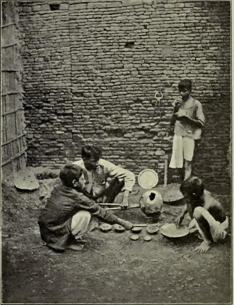
THE FURNACE : THE ARTISAN POURING THE MOLTEN KANSA INTO THE EARTHEN CRUCIBLES.
