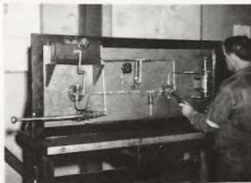
Mockup, Simple Hydraulic System.
