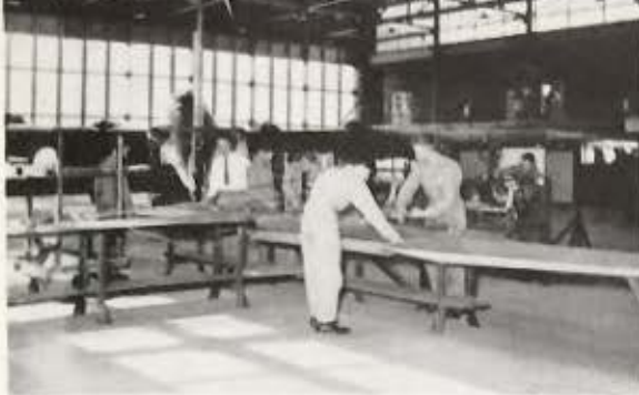
Repairing Wing Flaps.
