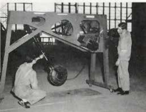
Mockup, Warning and Limit Switches System.
