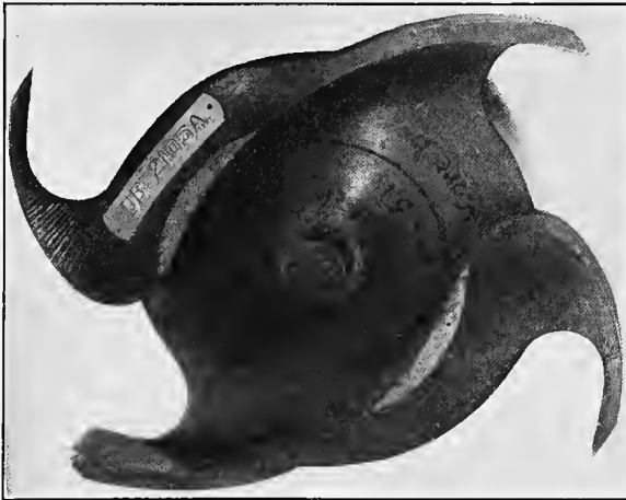
FIG. 277.—Impeller of Worthington trash pump.
