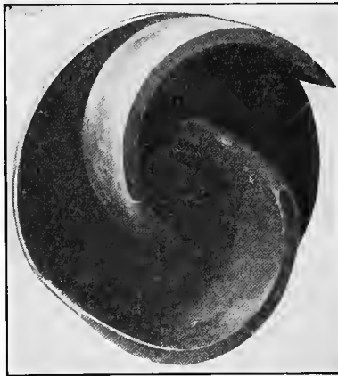
FIG. 273.—Impeller of Morris Machine Works non clogging pump.
