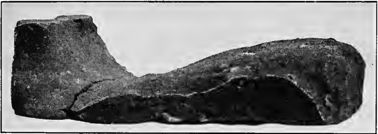
FIG. 146.—Brick forming manhole ledge.
