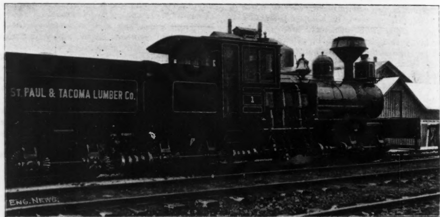
50-TON SHAY GEARED LOCOMOTIVE FOR THE ST. PAUL & TACOMA LUMBER CO. Lima Locomotive & Machine Co., Builders.
