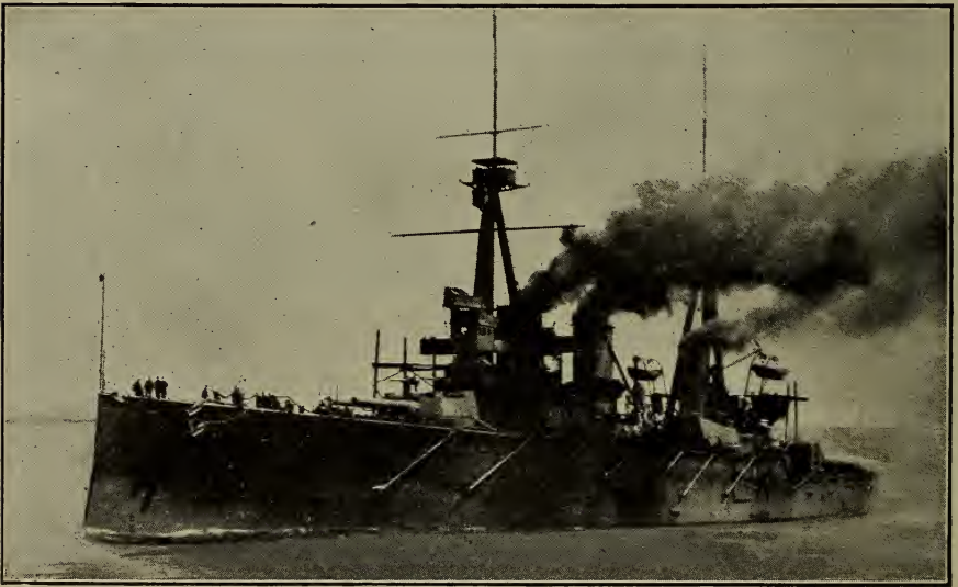
British cruiser "Indomitable." Length 560 feet, displacement 17,250 tons, speed 25 knots. She carries eight 12-inch and sixteen 4-inch guns.
