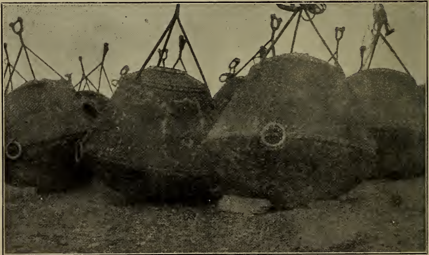
Mines taken from Kerr Bay, Nanshan, after the Japanese-Russian war. Mines are a part of the harbor defenses and are of many shapes and kinds, one of the most modern and successful of which is so arranged that when a ship strikes it an electric contact is made that notifies the operator within an armored casemate on the shore. If the vessel is a friend it is allowed to pass on, but if belonging to an enemy a switch is immediately thrown and the mine is exploded. Mines are so heavily loaded with high explosives that the explosion of one of them under a war-ship destroys the most powerful of them.
