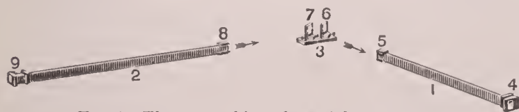
FIG. 4.—Elements of interferential comparator.
