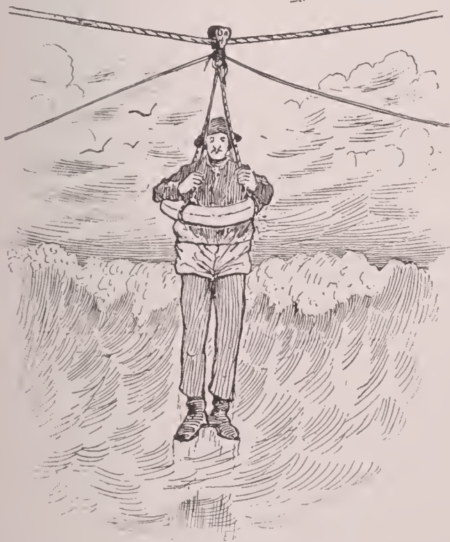
Method of using breeches-buoy.
