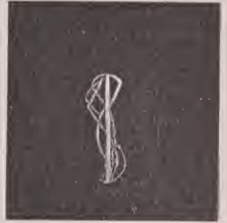
FIG. 10.—From photograph of an artificial oscillatory discharge in which several distinct paths are shown.
