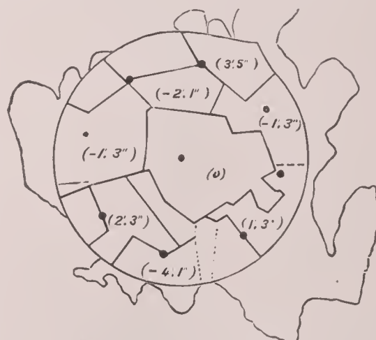
FIG. 2.—Minot's Ledge, as prepared to receive the foundation-stones.
