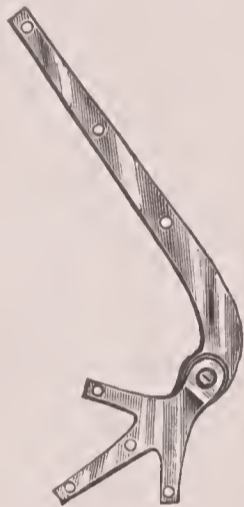
FIG. 9.—Showing a lateral knee-bearing joint iron.
