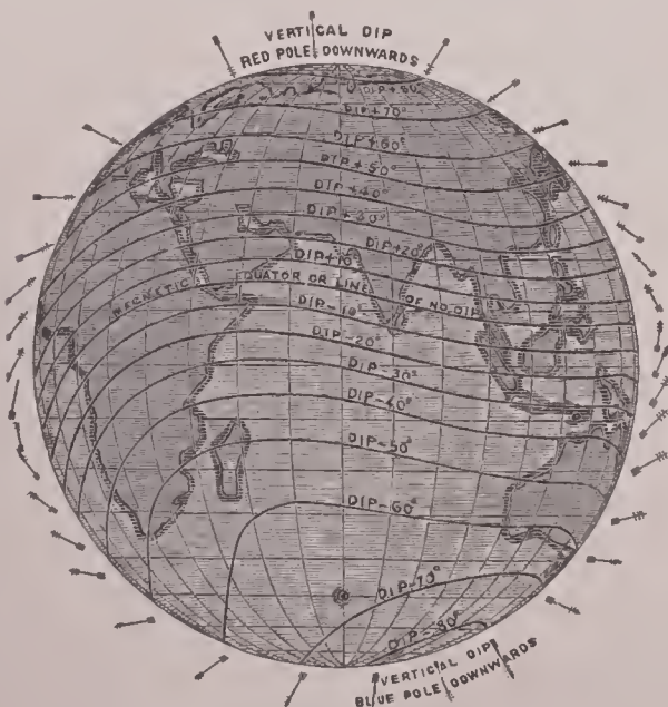
FIG. 5.—Magnetic dip and intensity.
