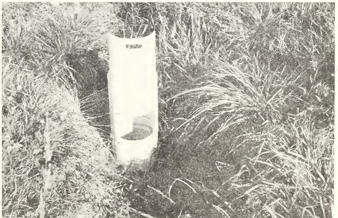
Figure 89.--Experimental risers initially installed on LeBeau's buried cablegation line. (Top) Swivel type with round outlets on each side and swiveling inner pipe. (Bottom) Slide type with rectangular outlets on each side.
