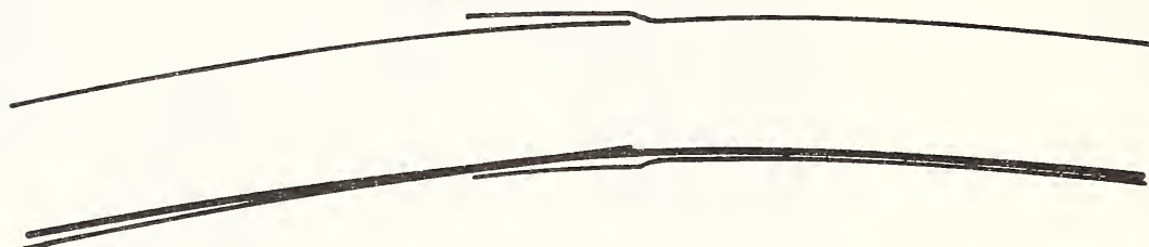
Figure 82.--Geometry of joints on curves which can cause the cable to groove or cut through the male end.
