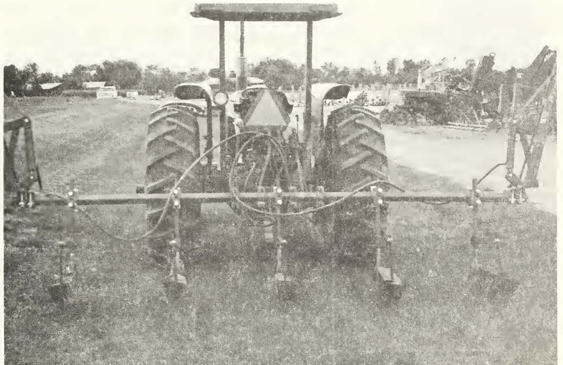
Figure 62.--Tractor and corrugator showing pattern of wheel compaction in corrugates responsible for differences shown in figure 52.
