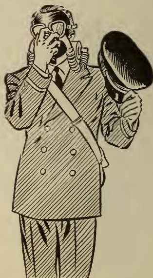
FIGURE 12.—Headgear removed with left hand. Mask removed from face by grasping diaphragm assembly with right hand.
