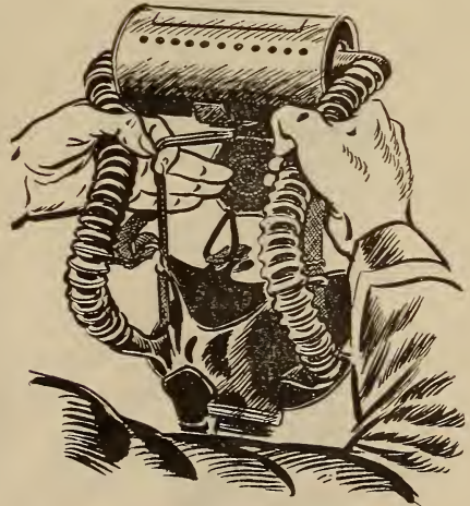
FIGURE 6.—Hoses and lower head harness straps encircled by thumb and first finger of each hand. Head pad raised by remaining fingers extended.
