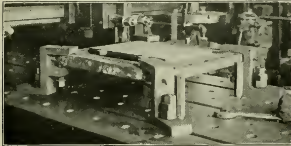
Fig. 1—Method of Planing Valve Chest Covers
