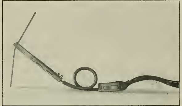
Welding Tool or Electrode Holder with Distant Control Switch
