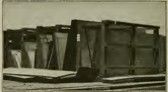
Rack for Storing Boiler Plate
