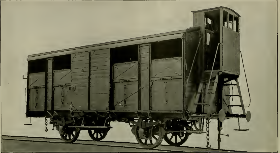
Fig. 2—View of the P. L. & M. Box Car, Showing Dropdoors in the Sides Open
