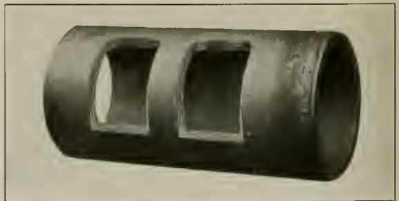
Three Sections of 8/4-in. Welded Steel Pipe Telescoped Without Failure
