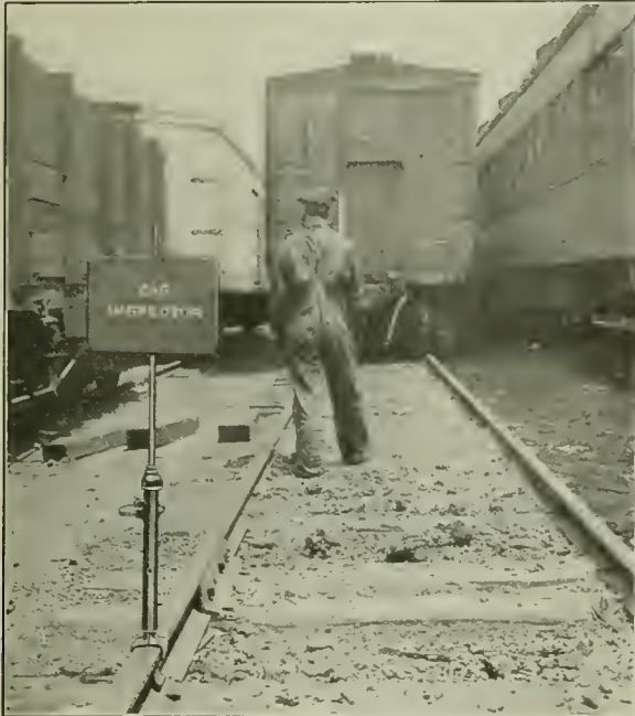
Blue Signal Safety Device Set in Position
