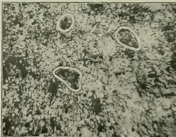
Fig. 2—Micrograph Showing Character of Pigment Particles of Brand No. 2 Magnified 150 Diameters
