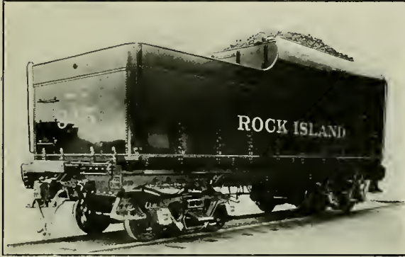
Rock Island Tender with Unusual Method of Joining Vertical and Bottom Tank Sheets
