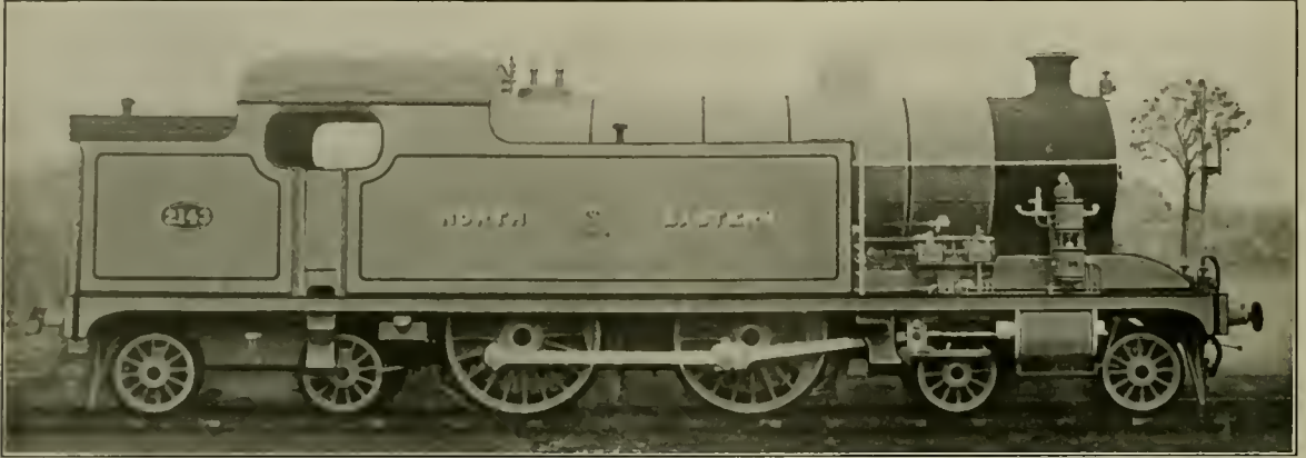
Three-Cylinder Tank Locomotive for Passenger Service, North Eastern Railway
