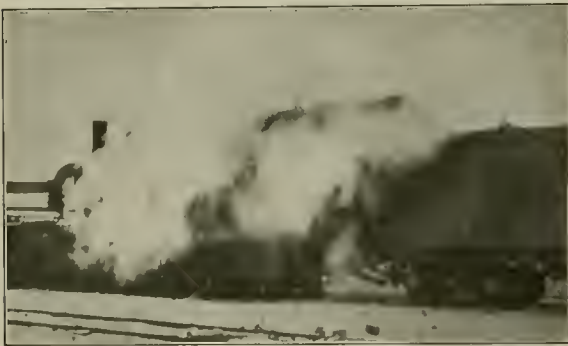
Steam Leaks Due to a Cracked Cylinder Found by the Government Inspectors
