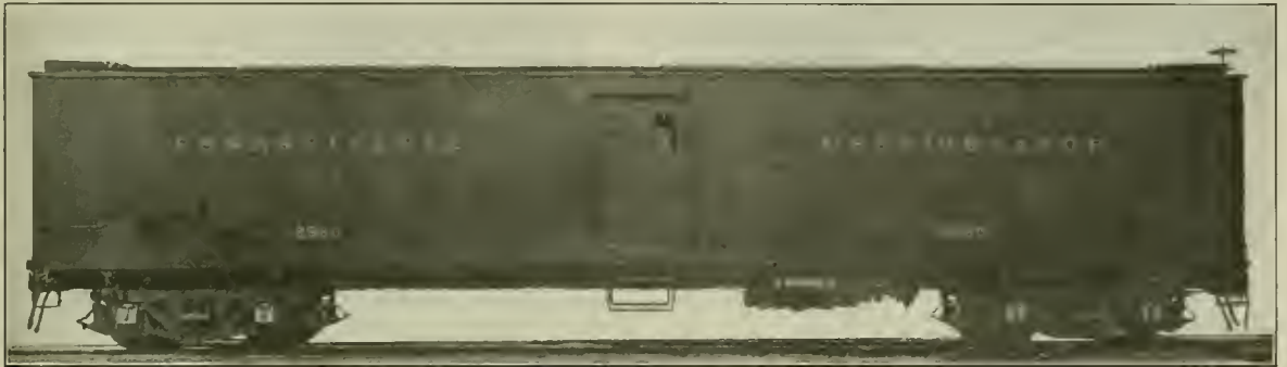
Refrigerator Car With Three Compartments for Rapid Loading
