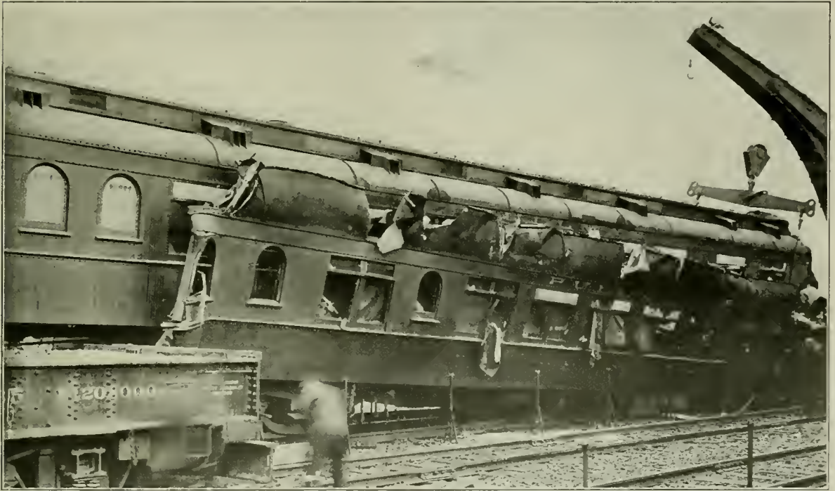
The Rear Car, Split Open and Telescoped by the Car Ahead
