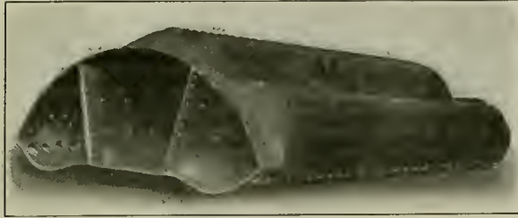
Steam Drums for the McClellon Firebox
