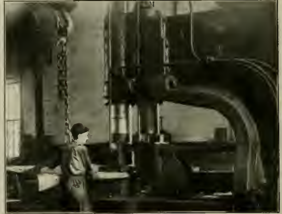
Fig. 1—Flanging a \frac{1}{2} -In. Tube Sheet Cold
