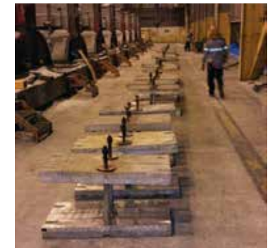
TOP LEFT: The anode baking equipment being removed from the bakes.
