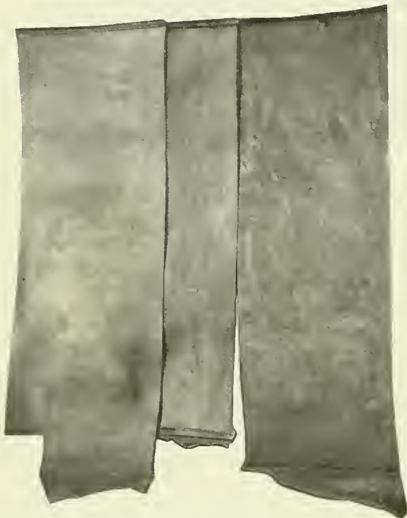
ILLUSTRATING DIFFERENCE IN STRETCH BETWEEN CENTRAL AND SIDE PORTIONS OF BELTING BUTT.
