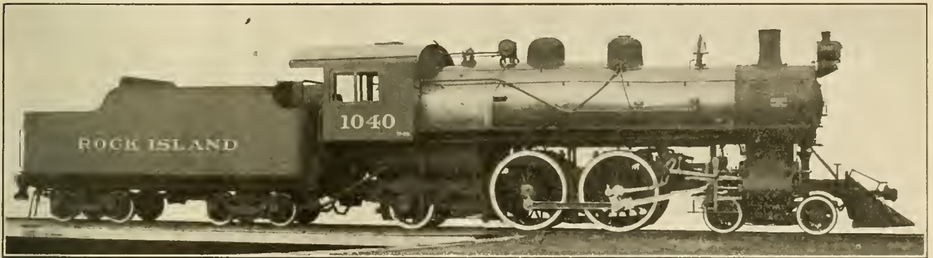
BALANCED SIMPLE ATLANTIC TYPE LOCOMOTIVE WITH SUPERHEATER—CHICAGO, ROCK ISLAND AND PACIFIC RY.
