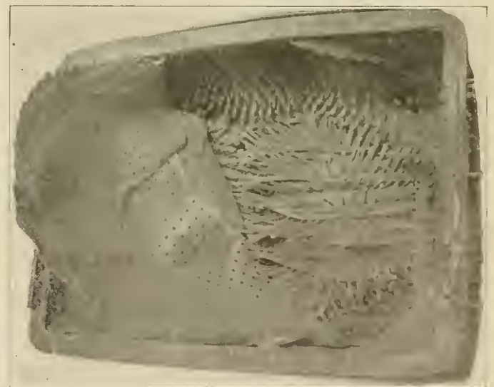
FIG. 5.—RUPTURED CROWN SHEET.
