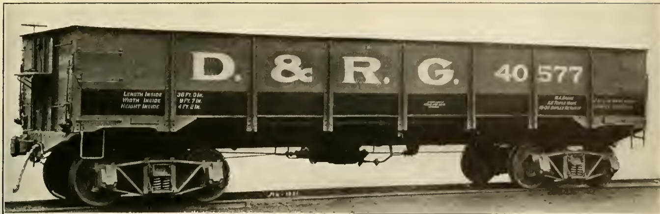
GENERAL SERVICE 50 TON, 36-FOOT STEEL CAR—DENVER & RIO GRANDE RAILROAD.
