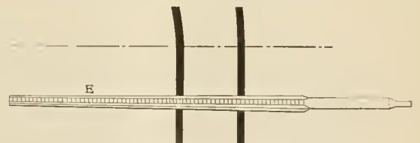
TAPPING HOLES IN A LOCOMOTIVE BOILER.
