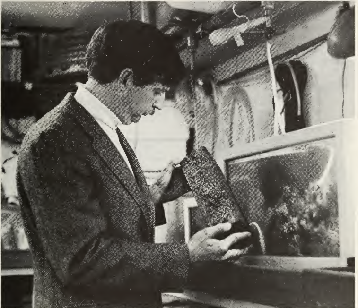
Students examining timber that has been infested with shipworms
