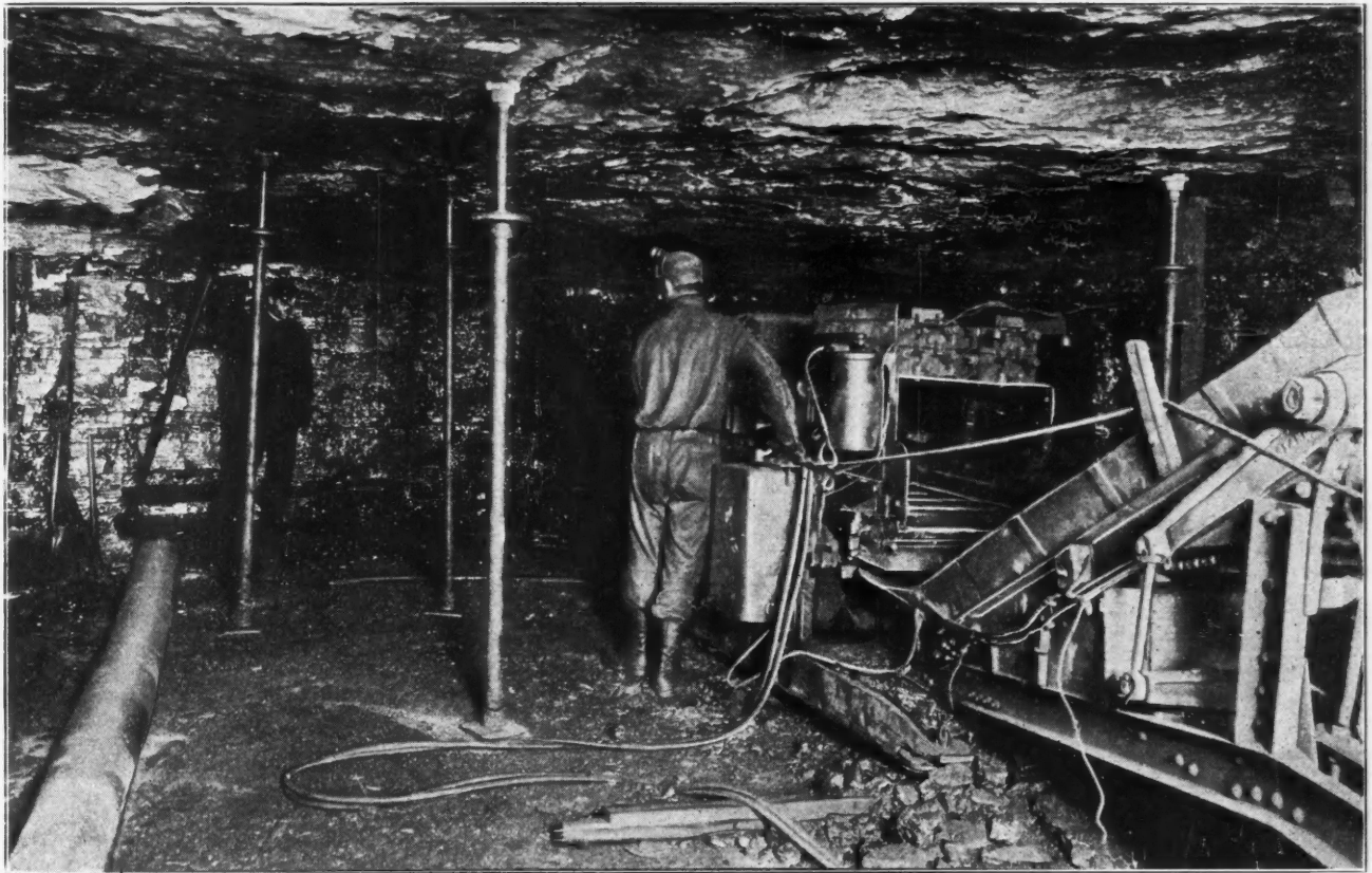
FIG. 9. JEFFREY-MORGAN MINING AND LOADING MACHINE
