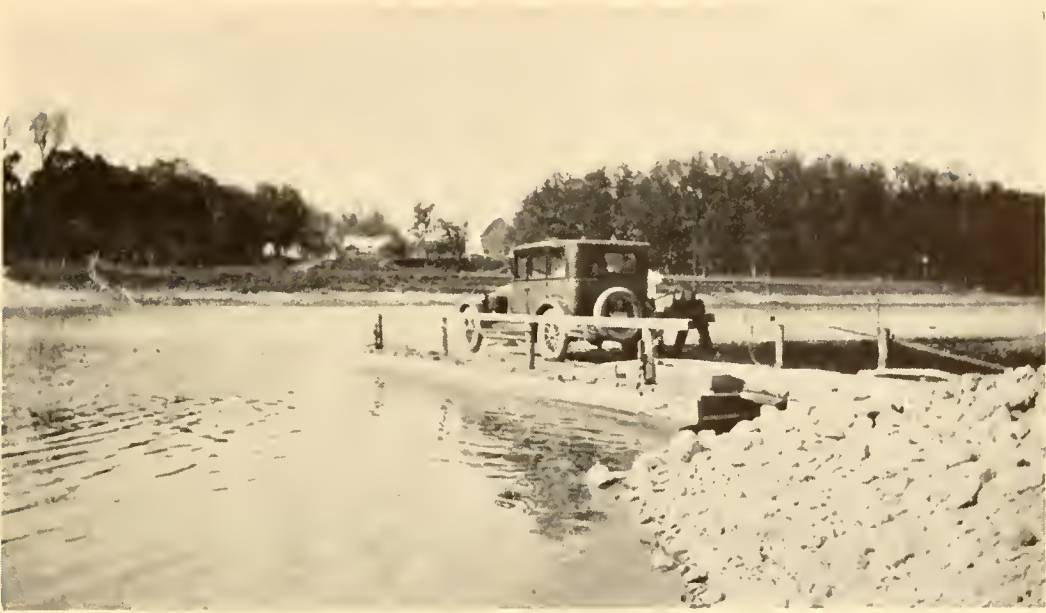
FIG. 179.—A ferry-float across the Grand River on the Six Nations Indian Reserve; it is propelled by the hands turning a toothed wheel over which passes a chain fastened to the shore, at either end.
