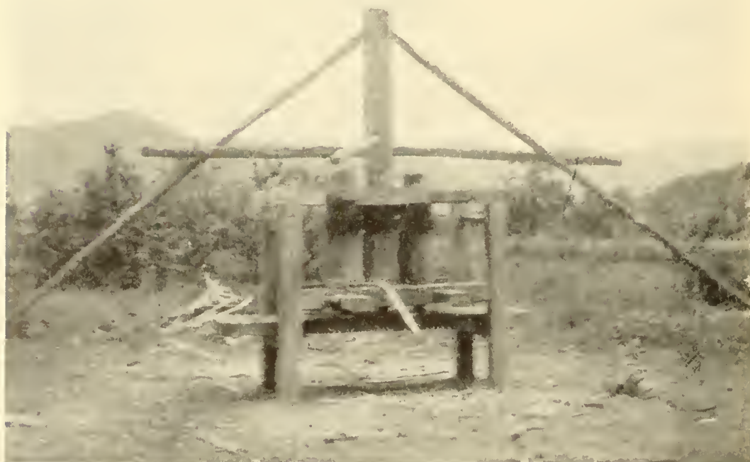
FIG. 127.—Three-roller sugar mill, Valley of the Rio Tiroo.
