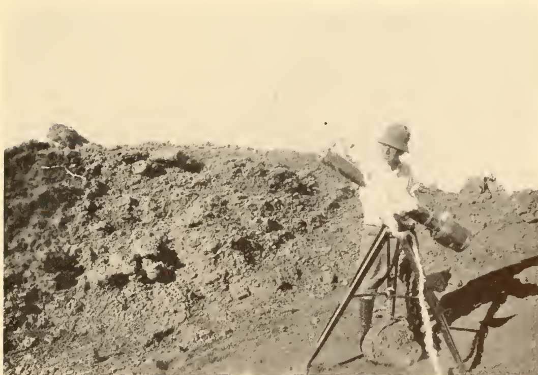
FIG. 4.—The new instrument at Fogo. Close-up view of Mr. Moore with the combination instrument for measuring atmospheric humidity, brightness of the sky, and intensity of solar radiation.
