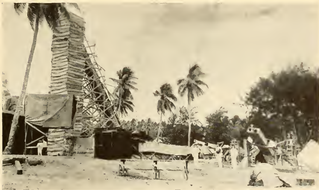
FIG. 60.—General view of the astronomical camp, showing the 63-foot direct view camera, the 65-foot reflecting camera, and the Einstein double camera on the right. (Photograph by Kellers.)
