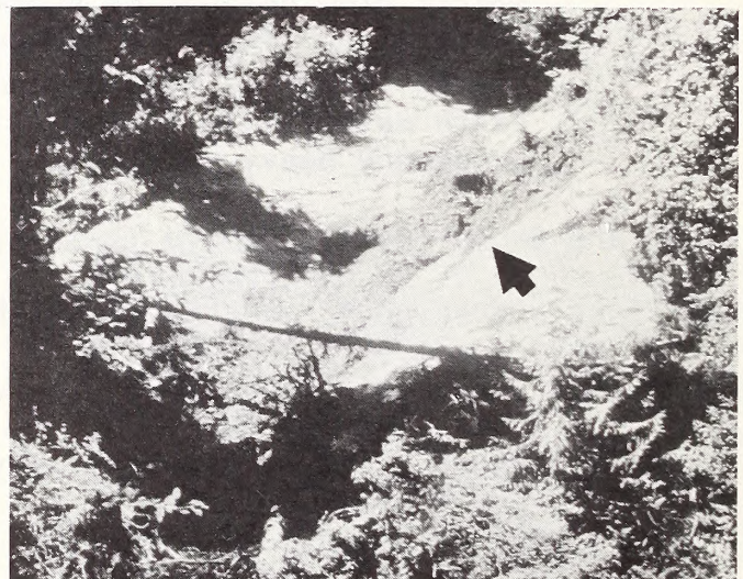
Figure 43 (below). The arrow shows loose material, dark with ground water.
