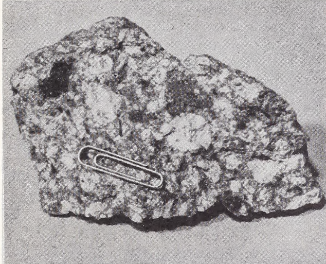
Figure 12. Volcanic breccia with coarse, angular fragments 1/4" to 2" in size
