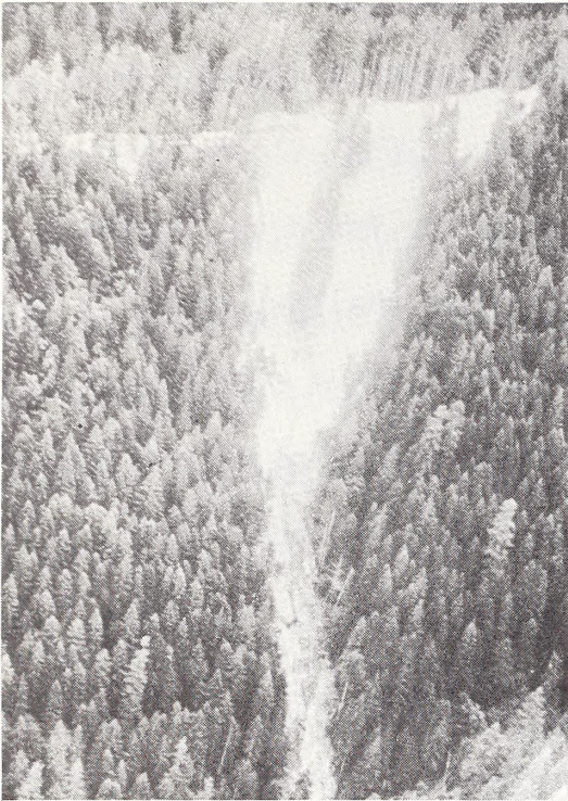
Figure 40 (left) and Figure 41 (above). These are two examples of debris avalanches in shallow soils on steep slopes.
