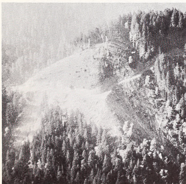
Figure 54. A photo of two steep headwalls where sidecast material from roads can cause debris avalanches
