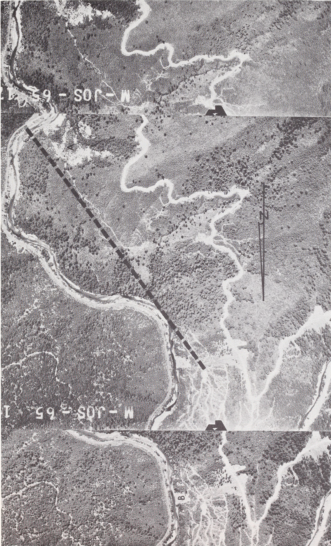
Figure 23. Stereogram of a possible fault zone. The location of the fault is indicated by the dashed line through the low saddle between the large, older slump at A and the newer slope failure at B.
