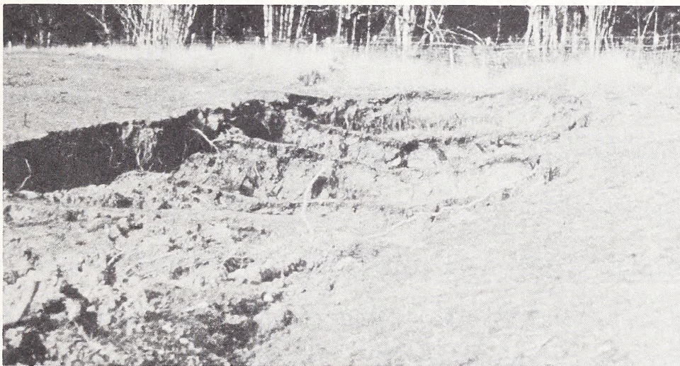
Figure 81. A progressive slump is a series of slope failures that may extend to the ridge top.
