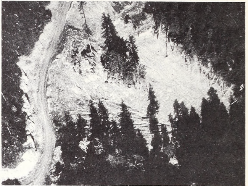
Figure 40 (left) and Figure 41 (above). These are two examples of debris avalanches in shallow soils on steep slopes.
