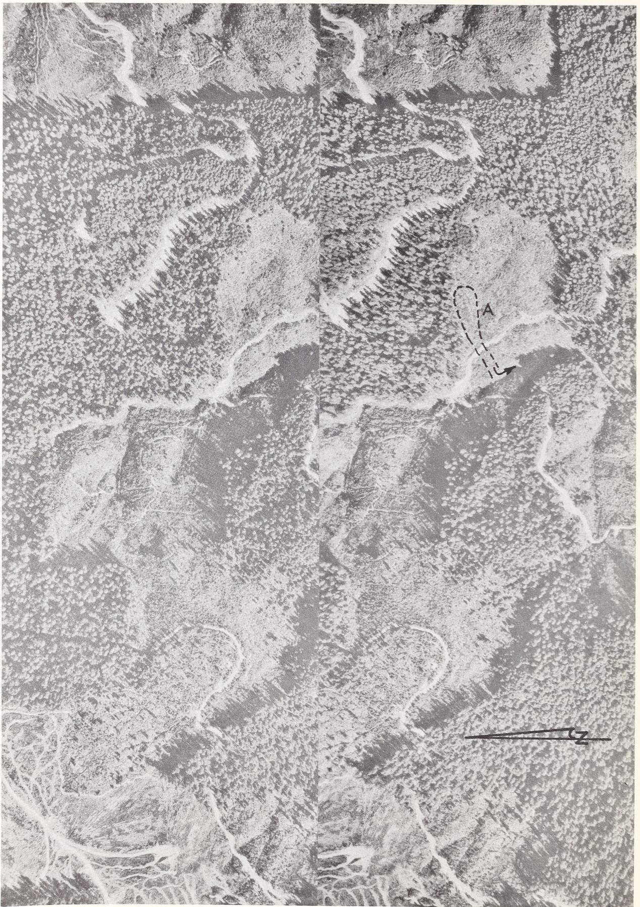
Figure 87. This stereogram shows unstable terrain derived from pyroclastic rock; there is evidence of active soil movement over the entire photo. An old slump is shown at point A and the dashed line outlines a new slump. Figure 88 shows a ground photo of this slump.
