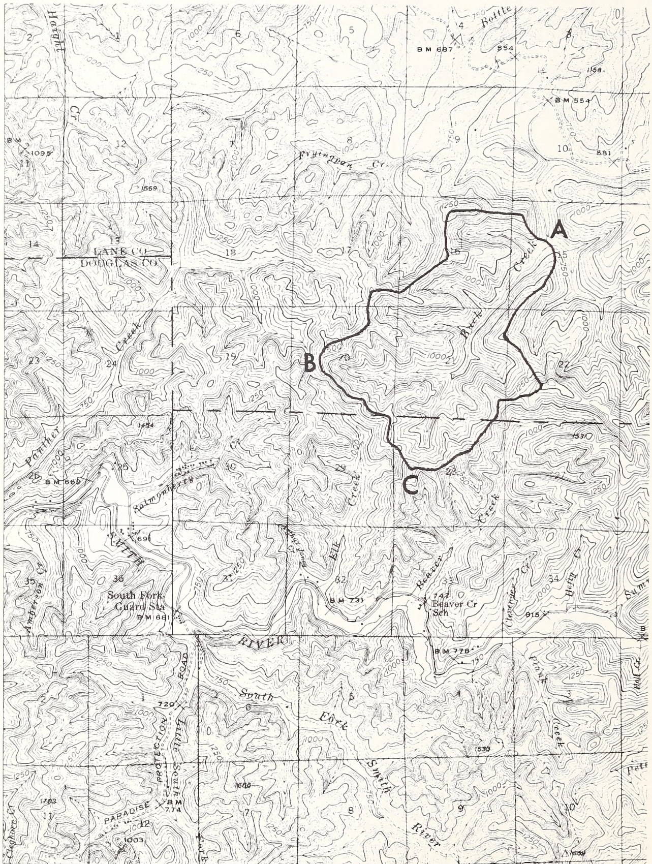
Figure 53. A topographic map of the steep terrain with sandstone bedrock where debris avalanches are the most common type of slope failure. The basin outlined in black is shown in the block diagram in Figure 52. Points A, B, and C may be used for orientation. Note the characteristic drainage pattern. Compare with Figure 66.
