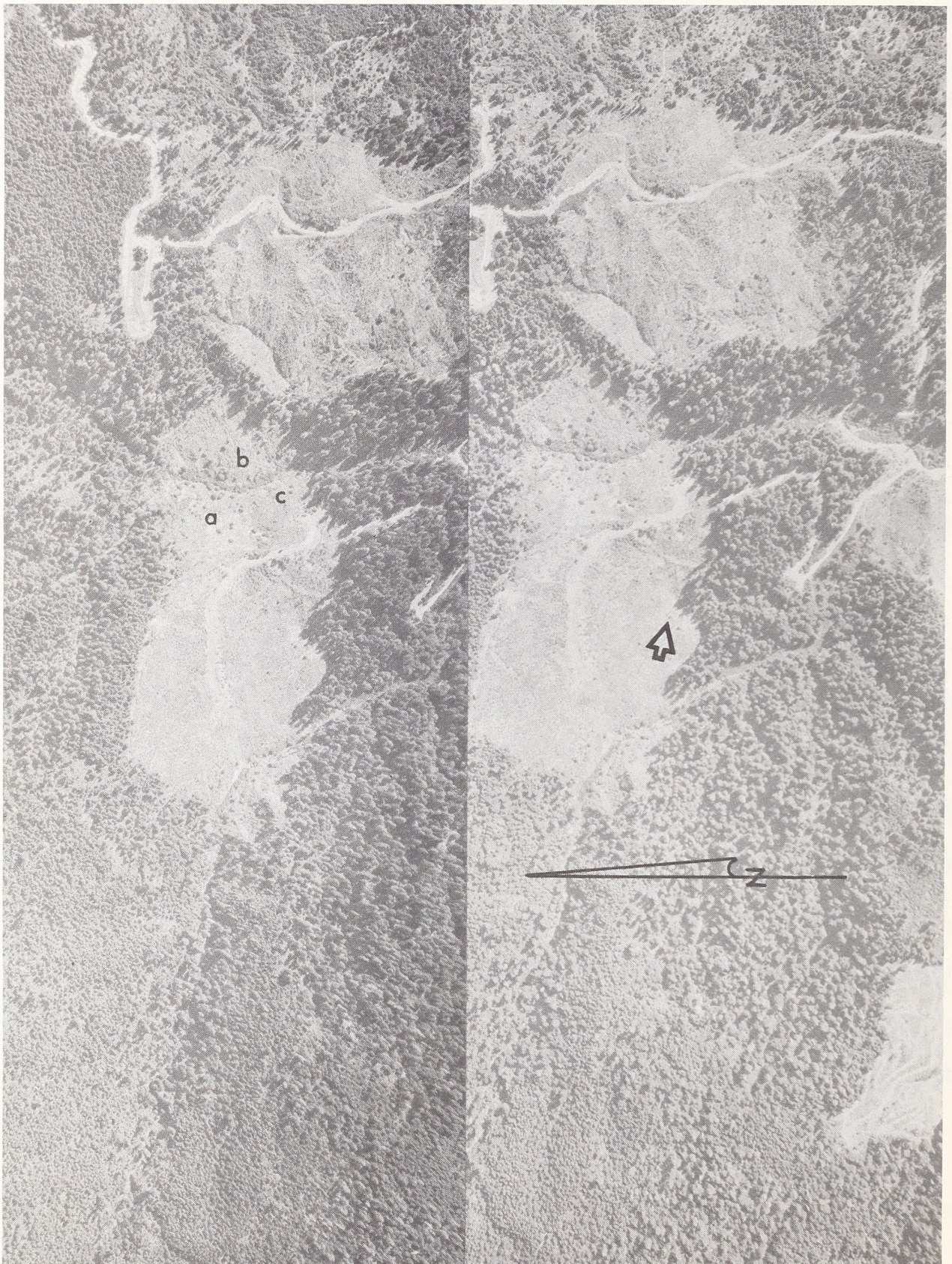
Figure 22. Stereogram of fault zone outlined in Section 27 of Figure 21. Large slump in center of photo; actively failing slopes at a and b. Arrow points to a dry sag pond below the slump.
