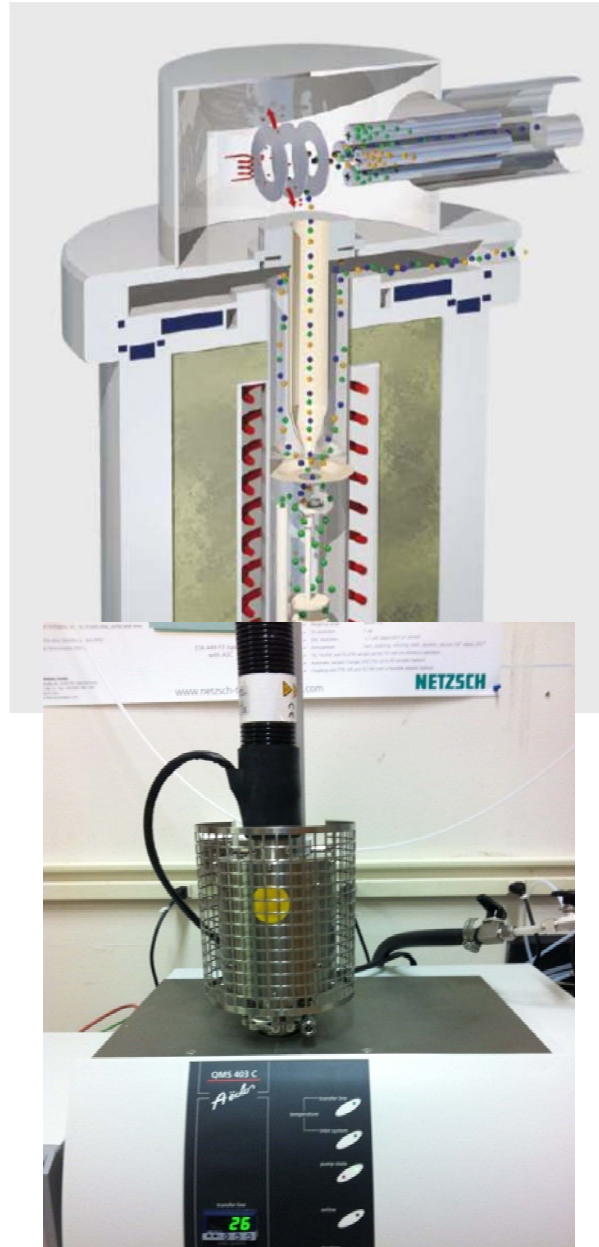
Figure 18. Diagram of the TA-QMS 403 Aëolos (left) (NETZSCH), picture of setup in NPS laboratory (right).
