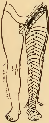
FIG. 104.—The Henry G. Davis hip-splint. Designed to give elastic traction; to give protection during locomotion, and to allow "motion without friction" at the hip-joint.
