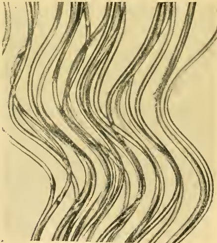
FIG. 4.—Artificial silk thread ( \times 80 ).
