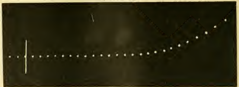
FIG. 6.—Record showing the latent period of Mimosa . The recorder vibrates 200 times per second. The time-interval between successive dots is here 0.005 sec.
