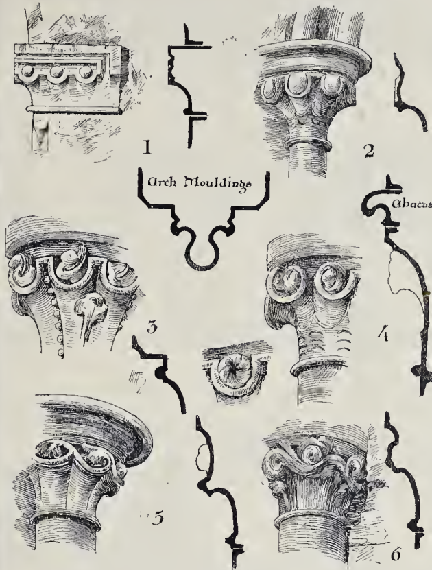
Deerhurst Church: Capitals in Nave, illustrating the Development of Gothic Foliage. Drawn by Mr. E. W. Collier.
