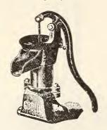
Fig. 205½ represents our Pitcher Spout Pump, with a closed top. It is often a cause of complaint with the Open Top Pitcher Pumps that they are apt to throw the water over the top when worked rather sharply. To obviate this, we have introduced a closed top with an opening only large enough for the rod to work through.
