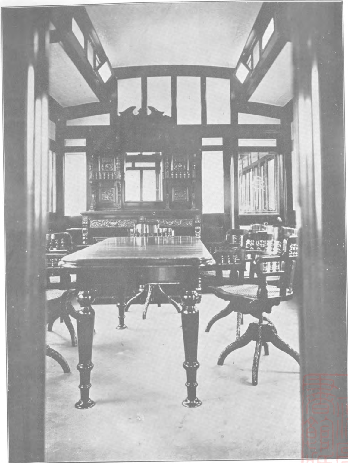
Interior of 1st class Saloon, fitted with teak wood sideboard, table, revolving chairs, ceiling covered with pegamoid, and floor with best "Cork Leno".
