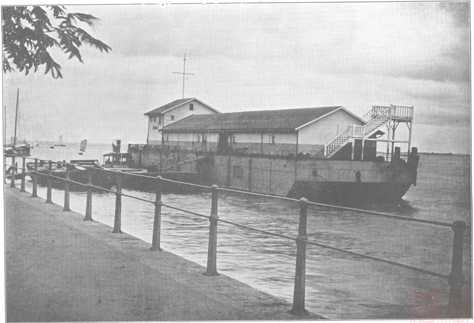
Steel Pontoon Hulk "Li Tai", built for Co Asiatique de Navigation, at Hankow. Dimensions 180' x 40' x 14' - Displacement 250 tons, Capacity 1750 tons, Deck houses, built of pine and hard wood, roof of galvanised iron sheets,
