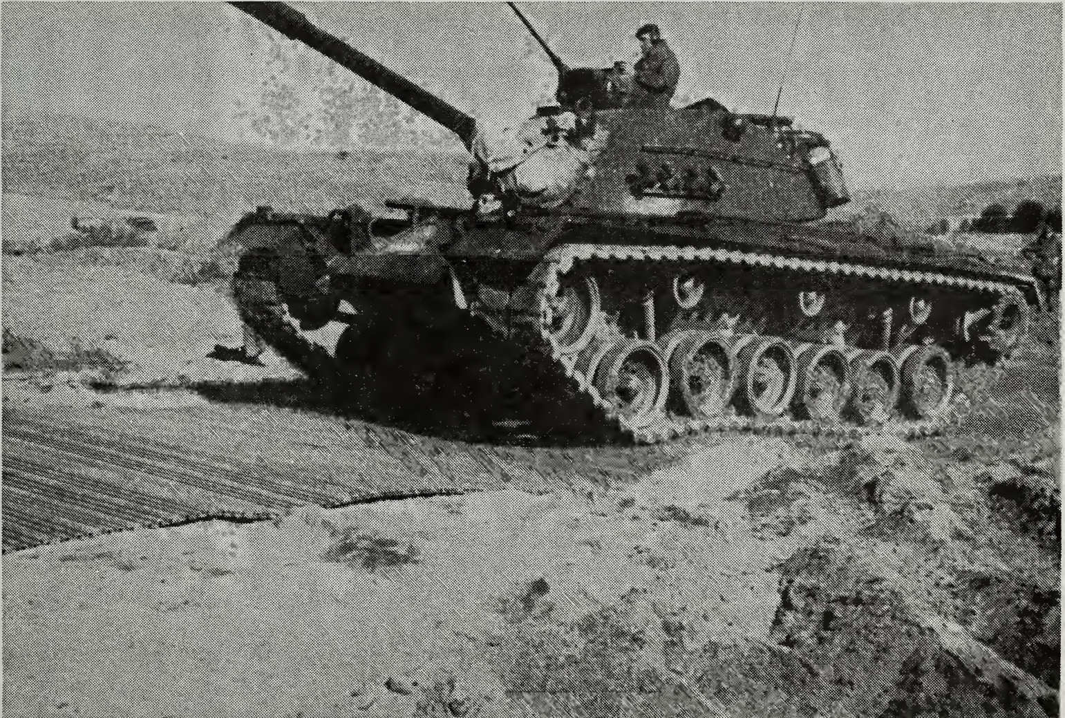
Figure 31. Class 60 Trackway System laid on sand in Middle East.
