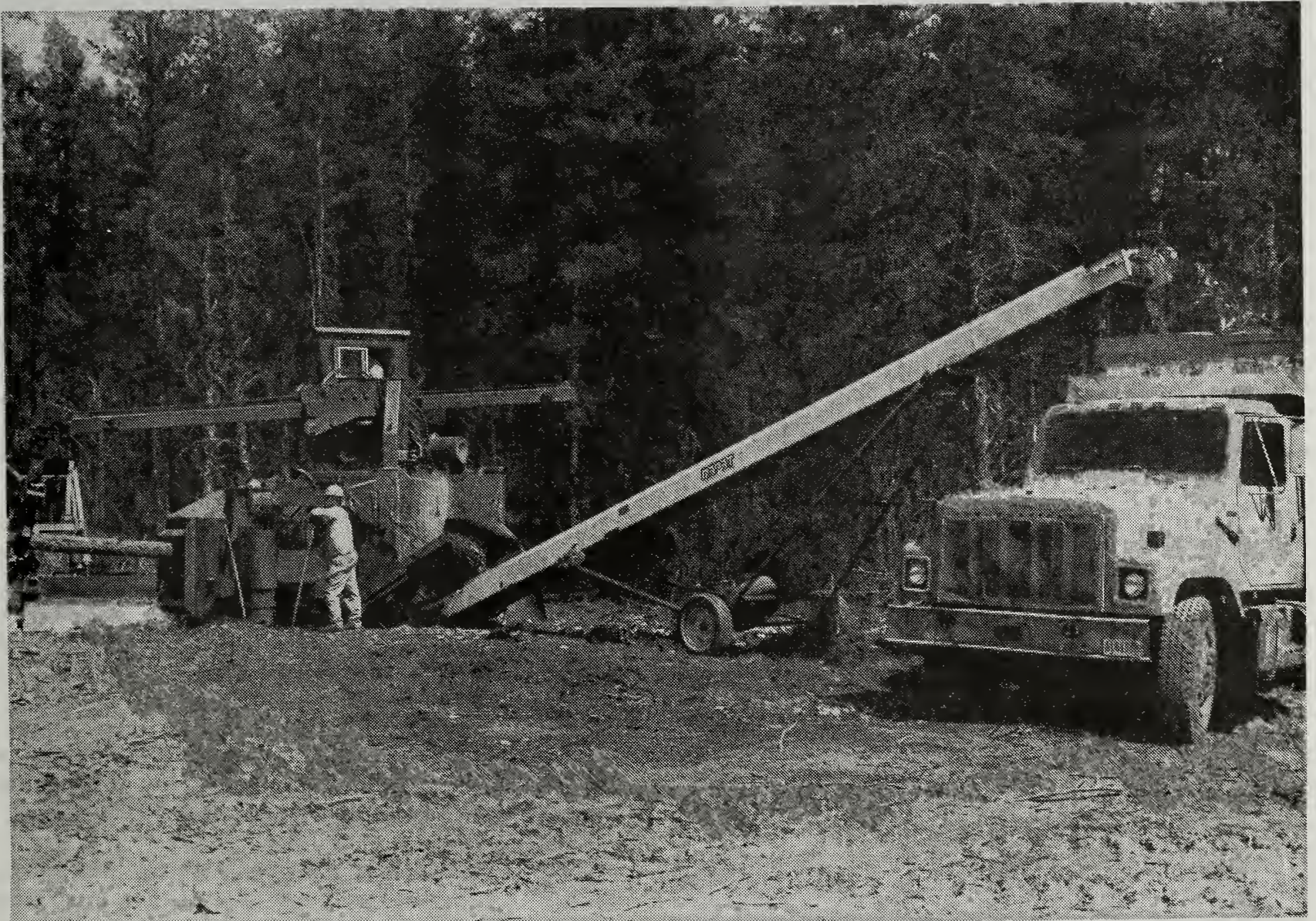
Figure 6. Chunkwood chunker machine in operation.
