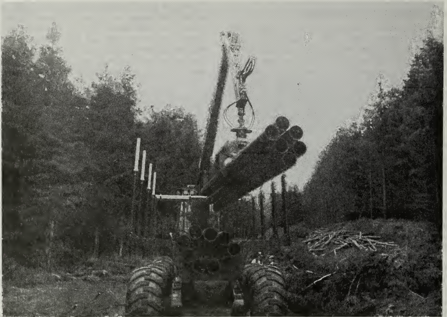
Figure 36. Transporting the Mini Pipe Fascine System.
