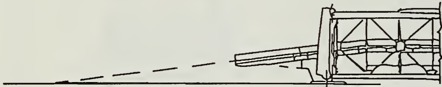
Elevation showing 3.05m (10') Timber Deck Ramp
