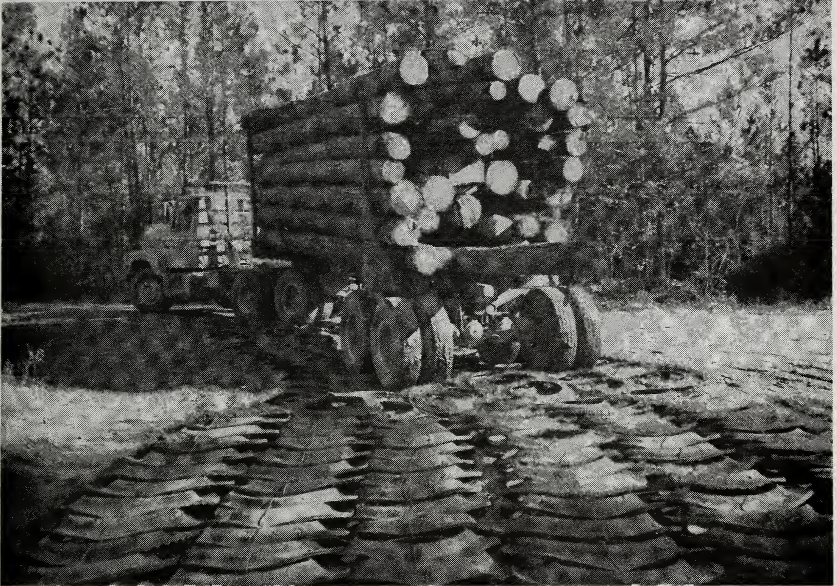
Figure 28. Rubber tires used without additional running surface.
