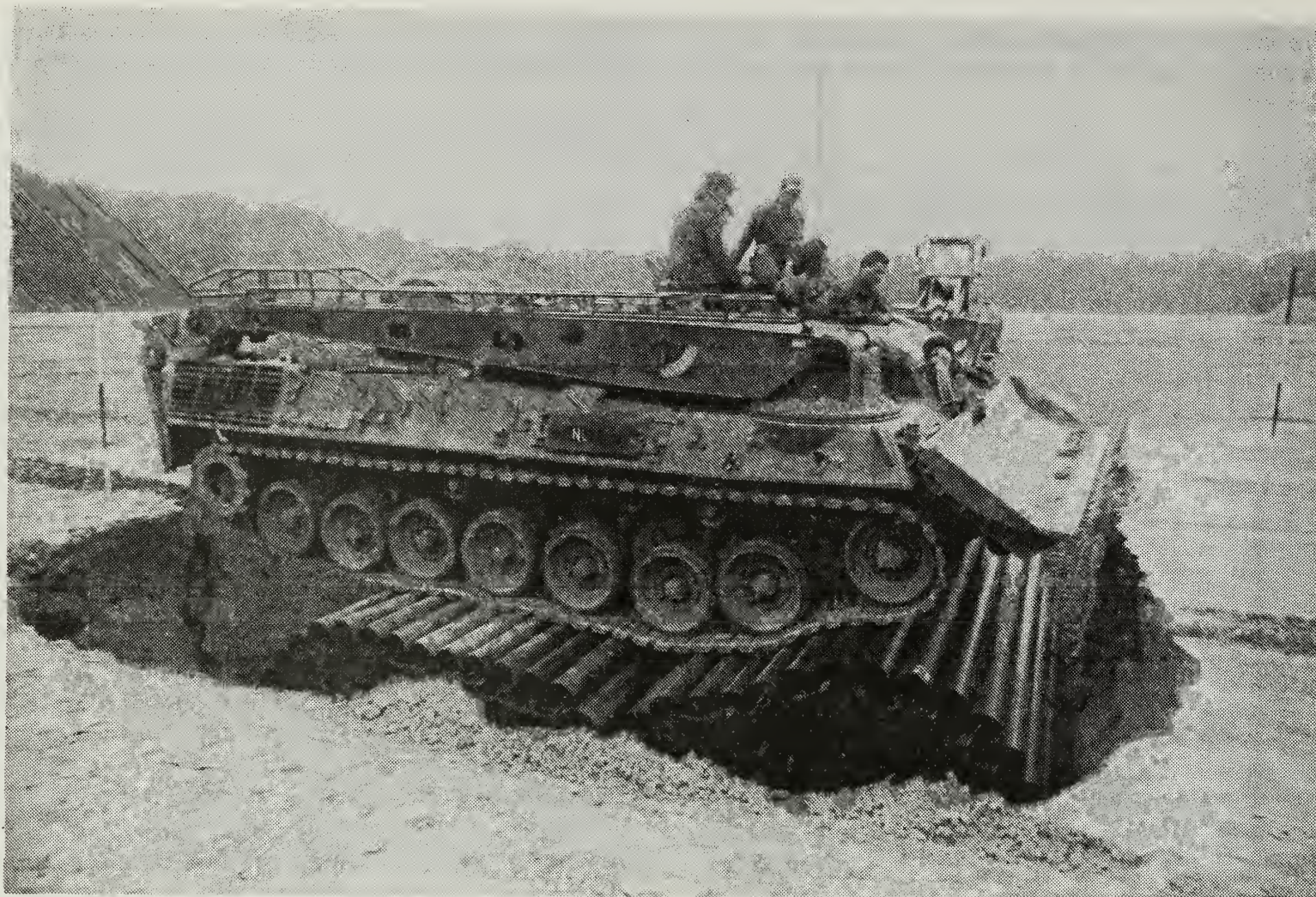
Figure 34. Pipe Fascine System used as fill material.
