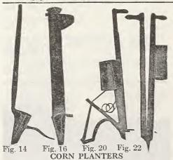
ACME AUTOMATIC—One Hand (Fig. 20)—Puts the right number of kernels just where you want them and at the proper depth, requiring only one hand, either right or left. Weight, packed, 6 lbs.
