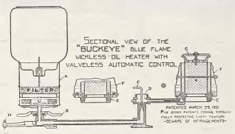
THE WICKLESS BURNER has a visible oil feed that is easily regulated and controlled. The oil container is glass and is outside of the hover—the oil being fed to the lighting ring in the center of the hover only as needed, and cannot become heated or ignited by the burner.
